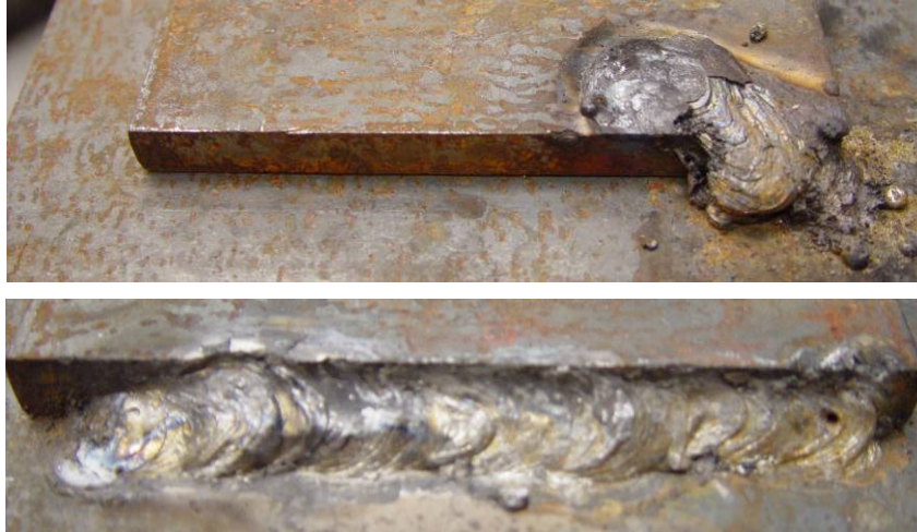
Figure 4.41: Specimen PC-5—Top Image-Incomplete Weld 1(Ice), Bottom Image-Weld 2(Ice)
