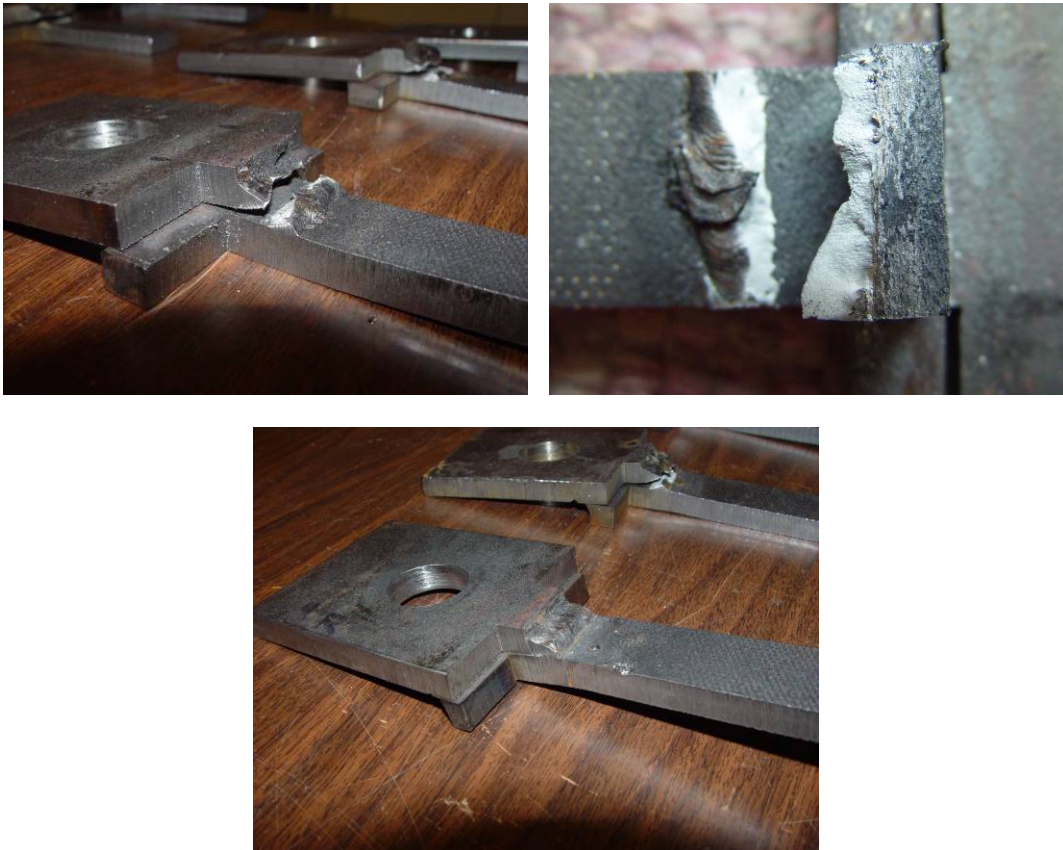
Figure 8.22: Post-test Specimen T-4
