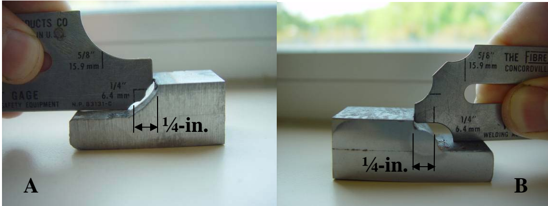
Figure 3.11: Fillet Weld Gauge—Concave Weld Measurement (A), Convex Weld Measurement (B)
