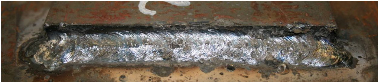
Figure 3.12: Example of Weld Classified as “Good” (1)
