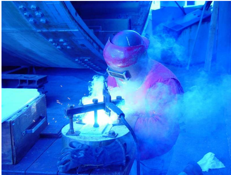
Figure 5.1: A36 Galvanized Specimen in Setup During Welding
