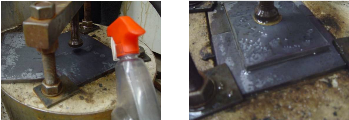
Figure 4.35: Wetting Process and Surface Wet Plate Assembly
