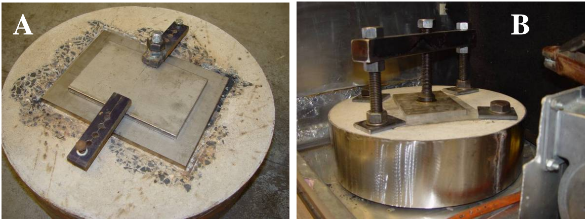
Figure 6.1: Stainless Steel Specimen in Setup: Original (A), Modified(B)
