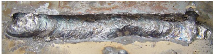
Figure 4.40: Specimen PC-4—Top Image-Weld 1(Wet), Bottom Image-Weld 2(Wet)
