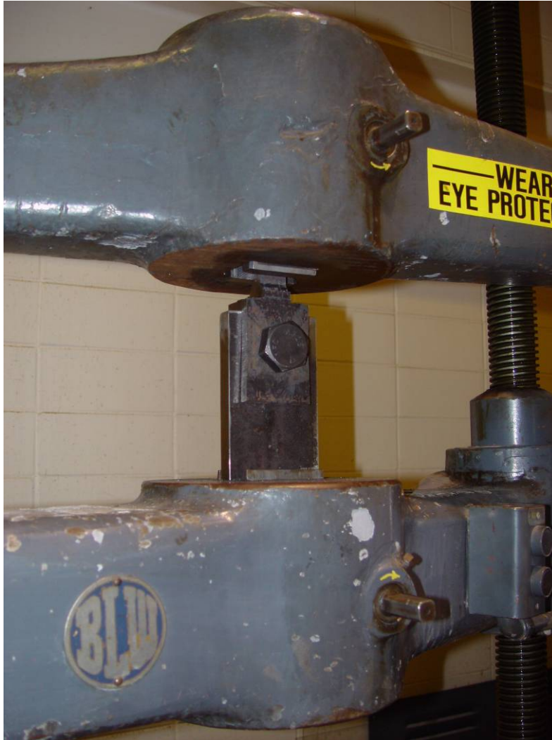
Figure 3.20: Tensile Test Apparatus and Loaded Specimen
