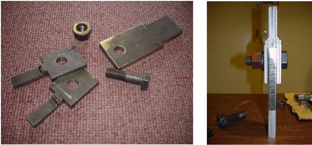
Figure 3.18: Complete Phase 2 Strength Test Specimen
