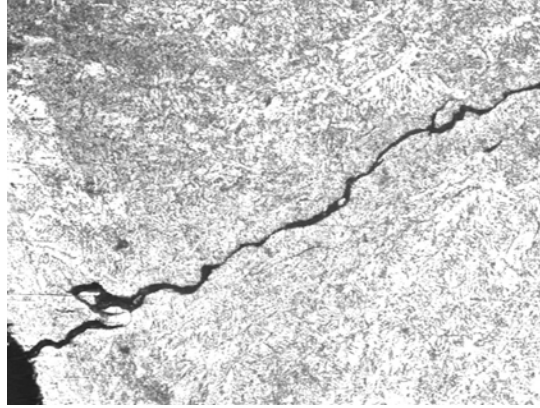
Figure 7.10: Solidification Crack in Specimen 36G-17HR
