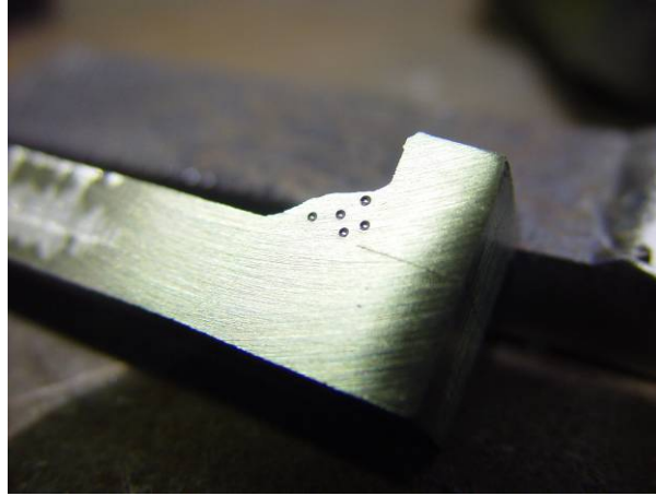
Figure 8.2: Rockwell B Hardness Indentations on Test Specimen Weld Cross-Section
