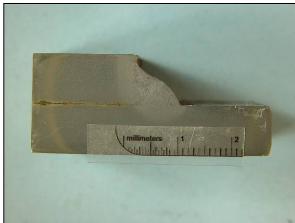
Figure 3.9: Polished A36 Cross Section
