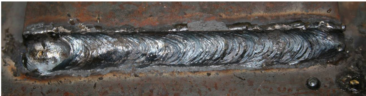
Figure 3.13: Example of Weld Classified as “Fair” (1)
