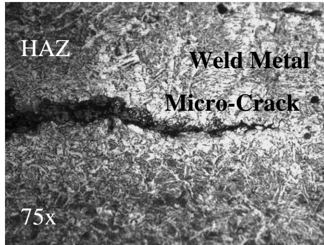
Figure 4.32: Micro-Cracking in Specimen 36-C2-Bottom-right Section
