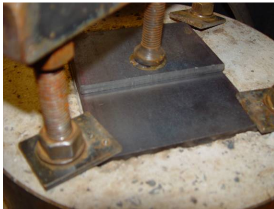
Figure 3.16: Phase 2 Strength Test Specimen in Concrete Block
