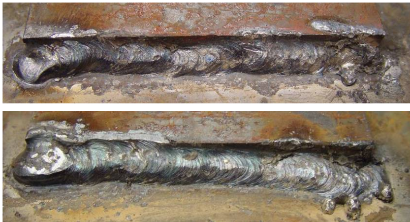
Figure 4.37: Specimen PC-1—Top Image-Weld 1(Wet), Bottom Image-Weld 2(Dry)
