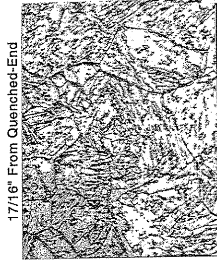
Figure 13 --- Steel H4 Jominy End Quenched Hardenability Microstructures - As Quenched
