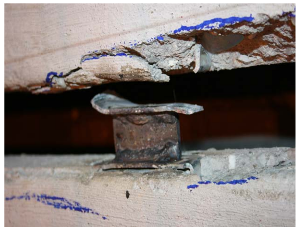
b) Half Scale Test of JVI Connector
