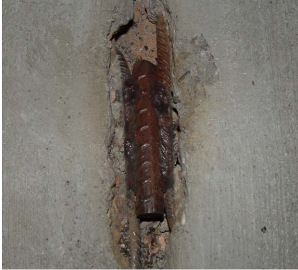
Figure 6-3: Half scale Topped Hairpin & Ductile Mesh Connector
