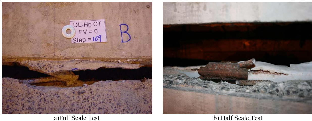
a) Full Scale Test b) Half Scale Test Figure 6-11: Failure Modes of Half and Full Scale Cyclic Tension Test of Topped Hairpin with Ductile Mesh Connector
