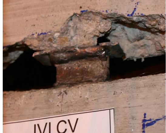
b) Half Scale Test of JVI Connector
