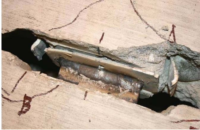
a) Full Scale Test of JVI Connector
