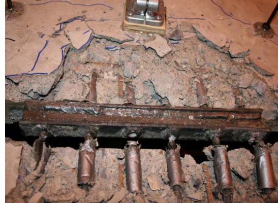
b) Half Scale Test of Unbonded chord Connector
