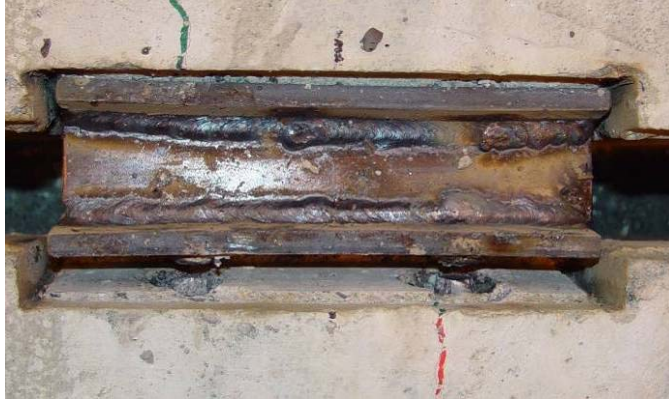
a) Full Scale Test of Unbonded chord Connector
