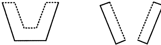
Figure 4: (a) Good Weld Pattern. (b) Poor Weld Pattern.
