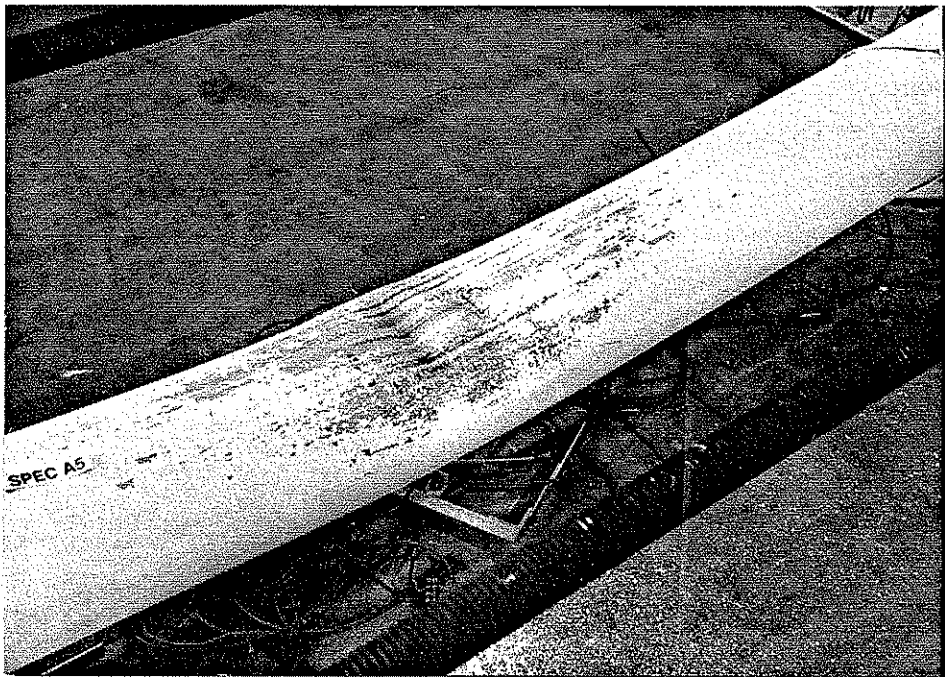
Figure 3.3. Formation of a local buckle on the compression face of Specimen A5.
