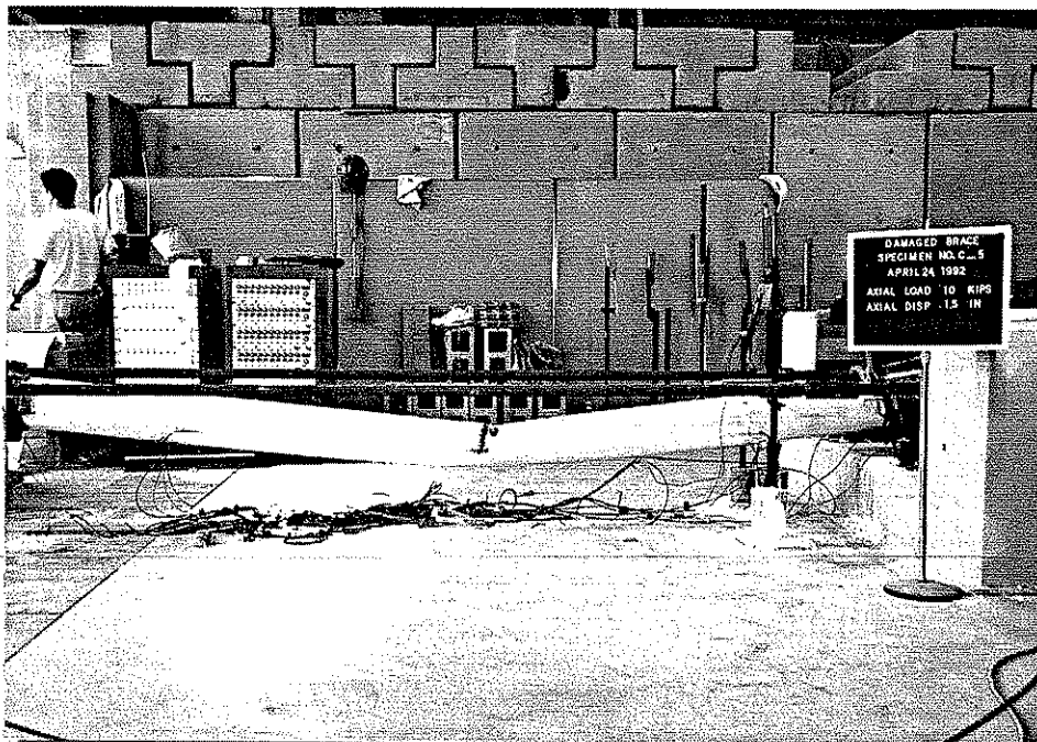
Figure 3.14. Corresponding in-plane displacement of Specimen C5 after continued shortening.
