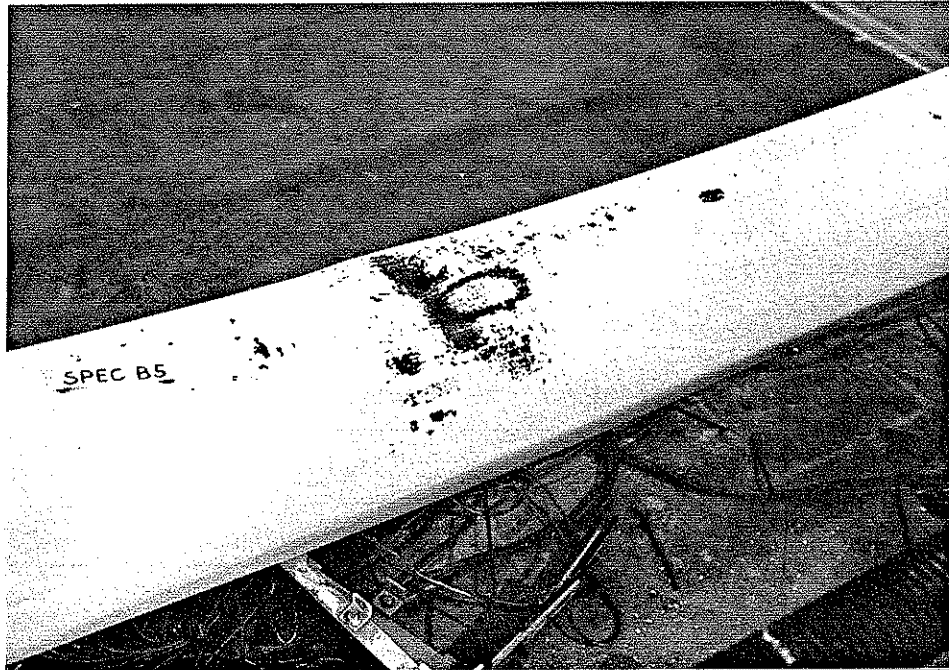
Figure 3.8. Formation of a local buckle on the compression face of Specimen B5.
