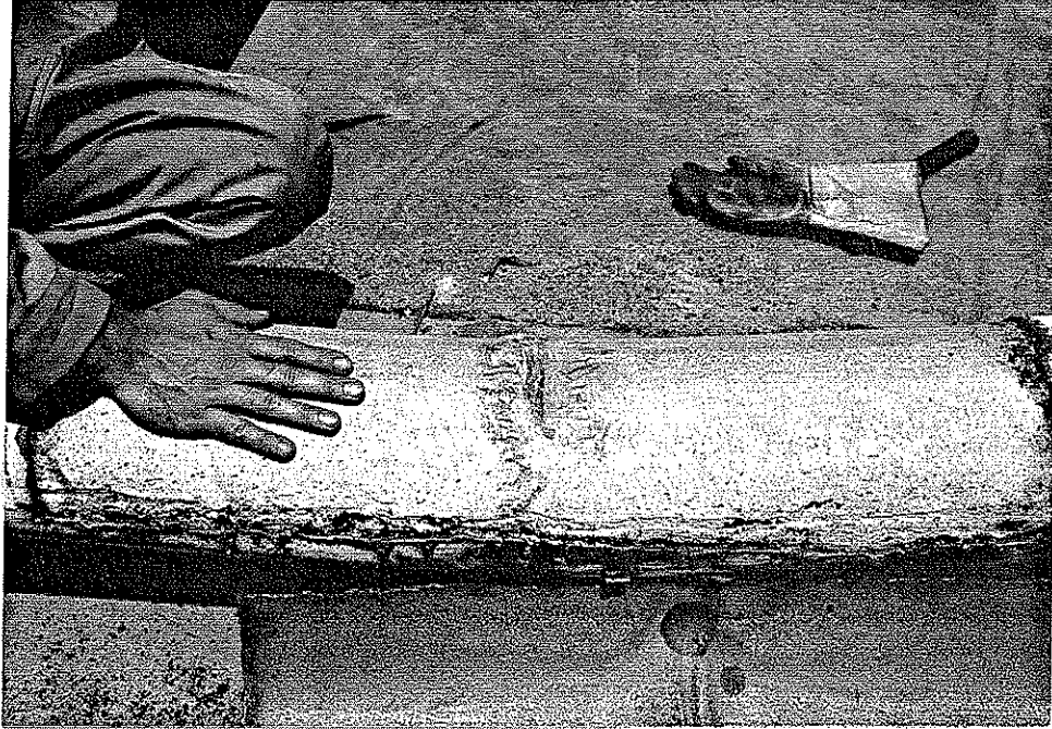
Figure 3.79. Exposed Grout Beneath Dent, Specimen C3.
