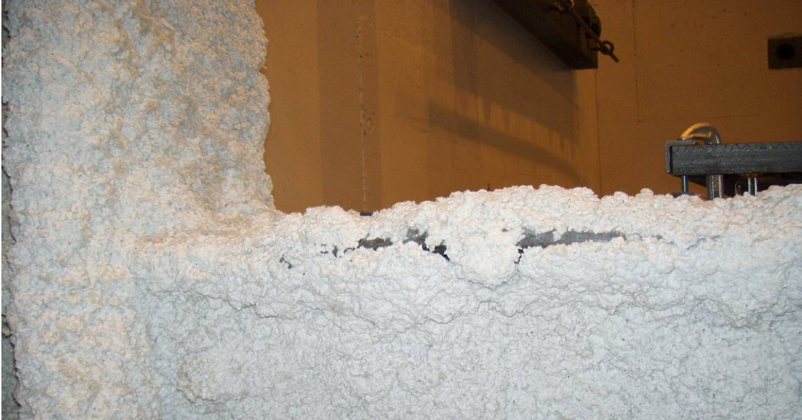
Figure 4.48 – Longitudinal splitting on top flange SFRM of DM assemblage during step 10
