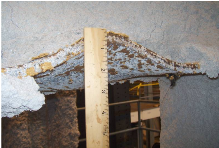
Figure 4.45 – Close-up of local buckling in bottom flange at completion of WM assemblage test
