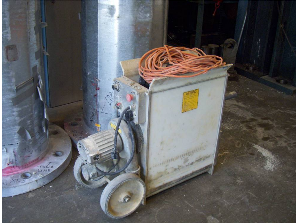
Figure 3.10 – Spray applicator for DM
