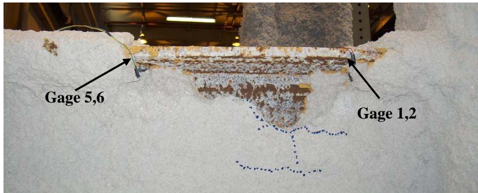
Figure 4.46 – Top flange of WM assemblage with gage locations at completion of test
