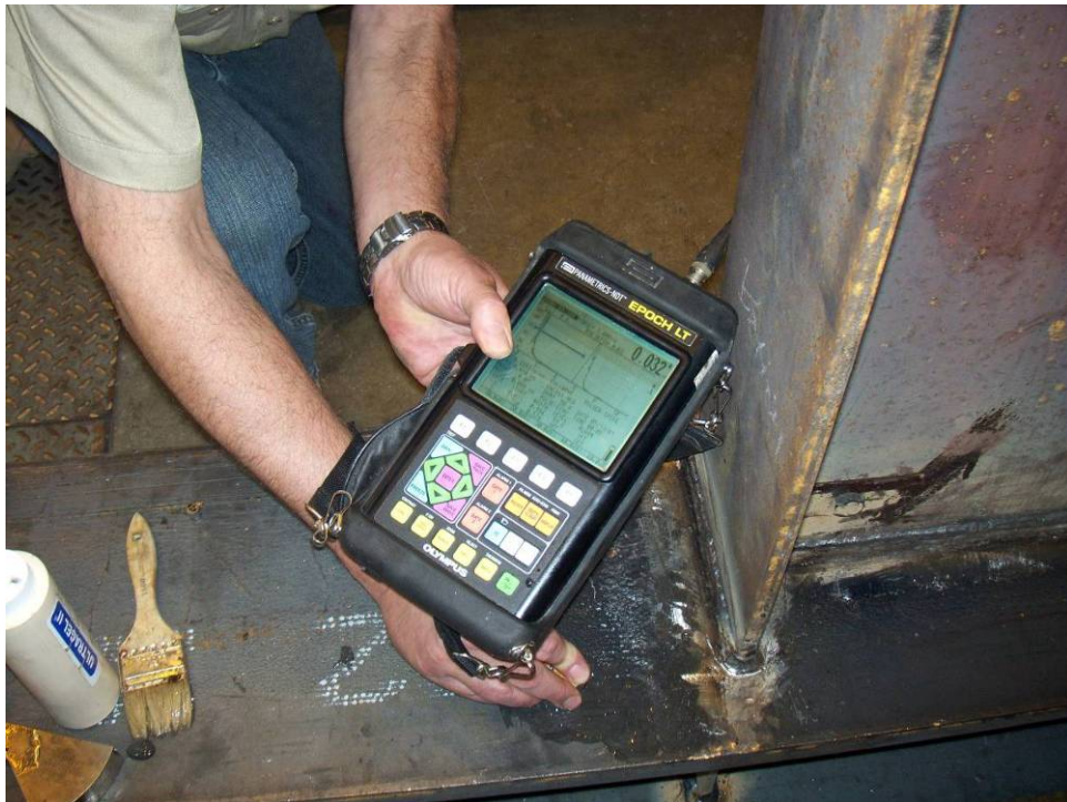
Figure 3.8 – Ultrasonic testing of specimen
