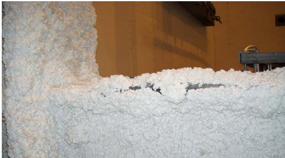
Figure 4.8 – Tear in top flange seen during step 10 of loading shown as Point B in Figure 4.6
