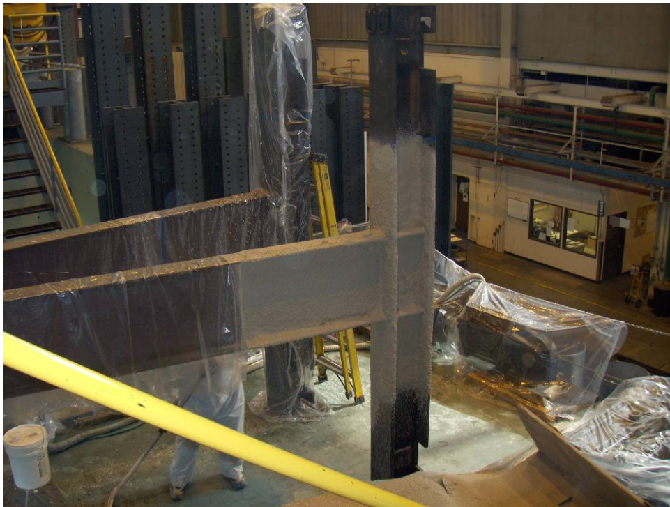
Figure 3.16 – Specimen after first coat of WM
