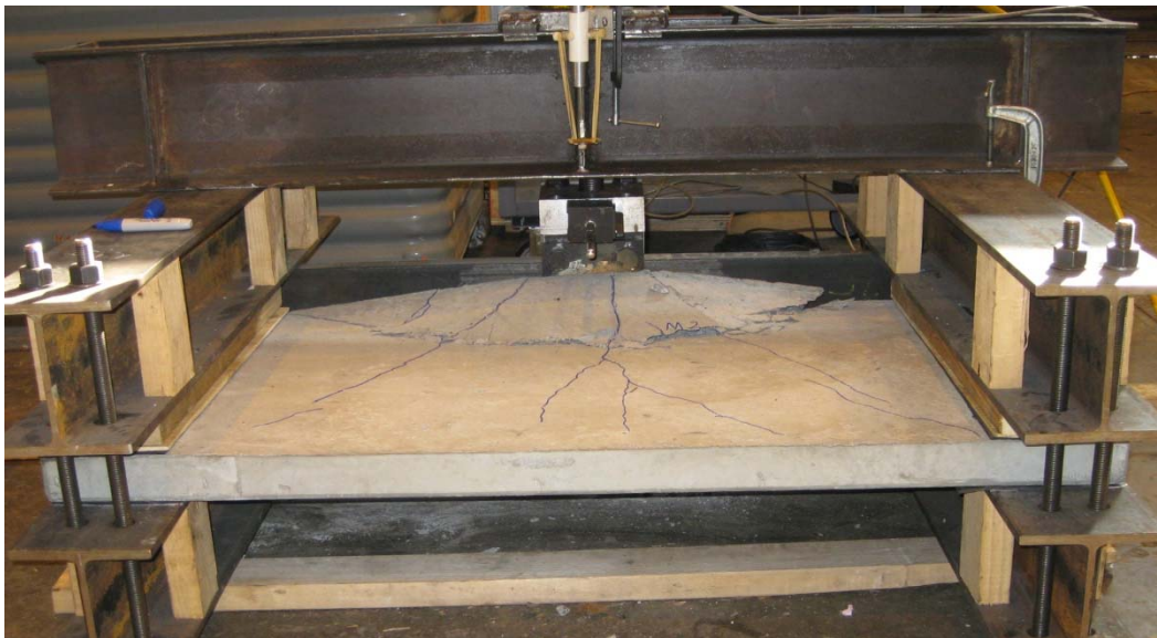
Figure 11: Damage at end of test OV2
