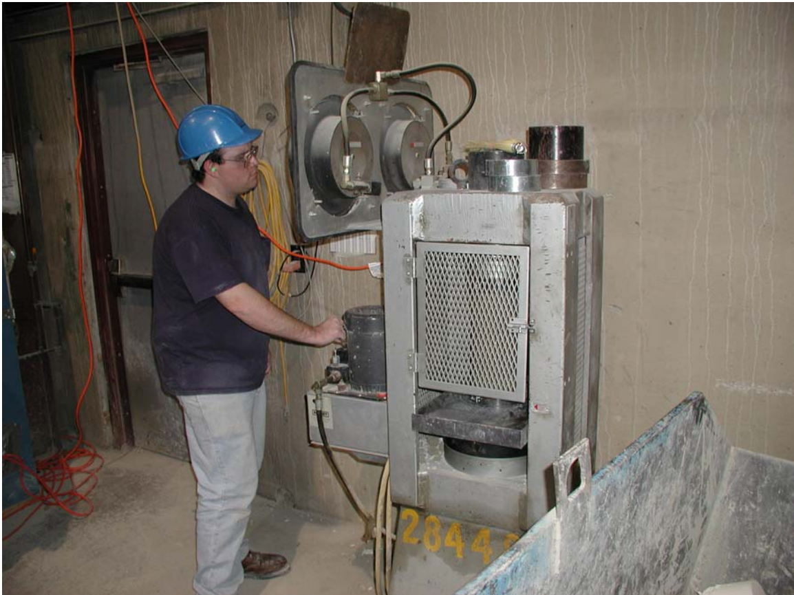
Figure 3.6 – Cylinder being tested in compression
