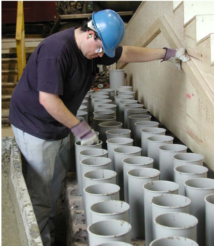
Figure 3.2 – Preparation of cylinder specimens in the precast plant
