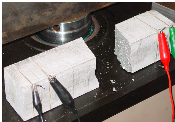
Figure 1: Brittle Fracture of Plain Mortar
