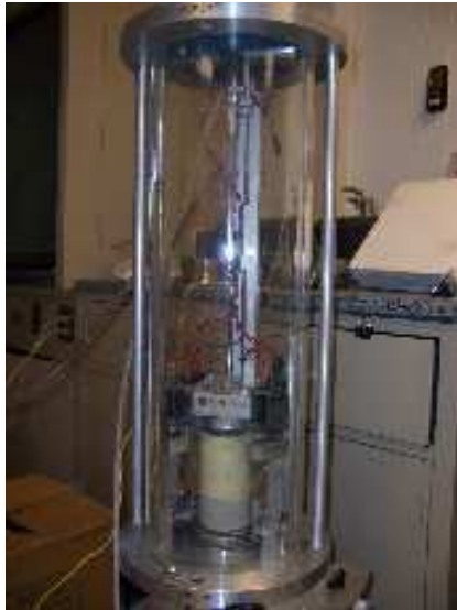
Fig. 2. Drenvich Longitudinal-Torsional Resonant Column
