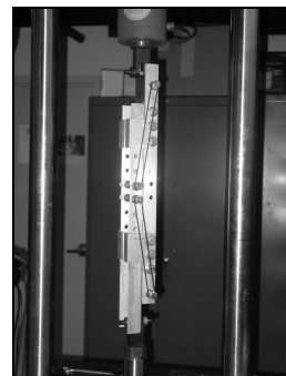
Figure 7. Superelastic SMA wires attached
