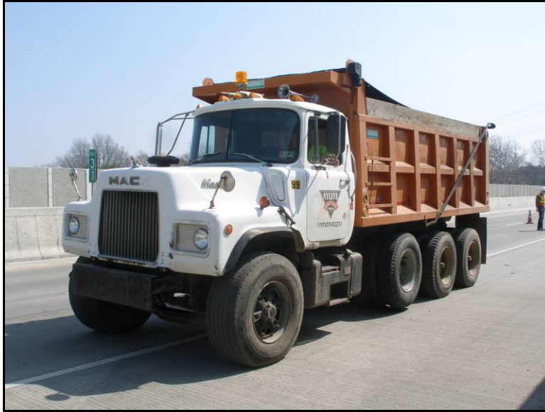
Figure 2.9 – Test truck used during controlled load tests
