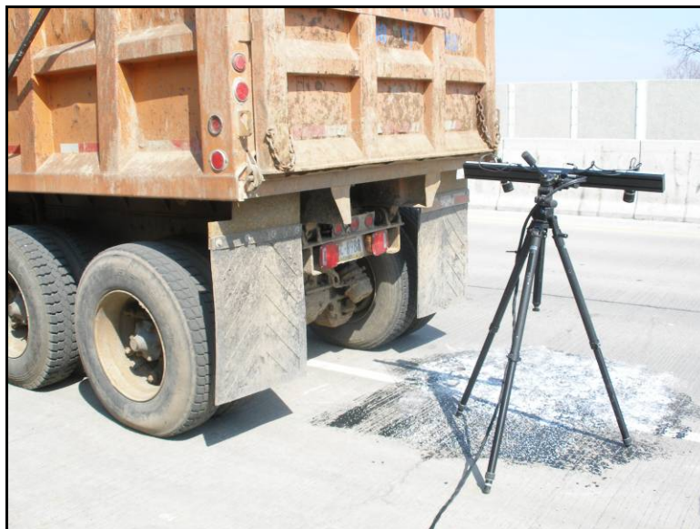
Figure 2.11 – Position of test truck during load test
