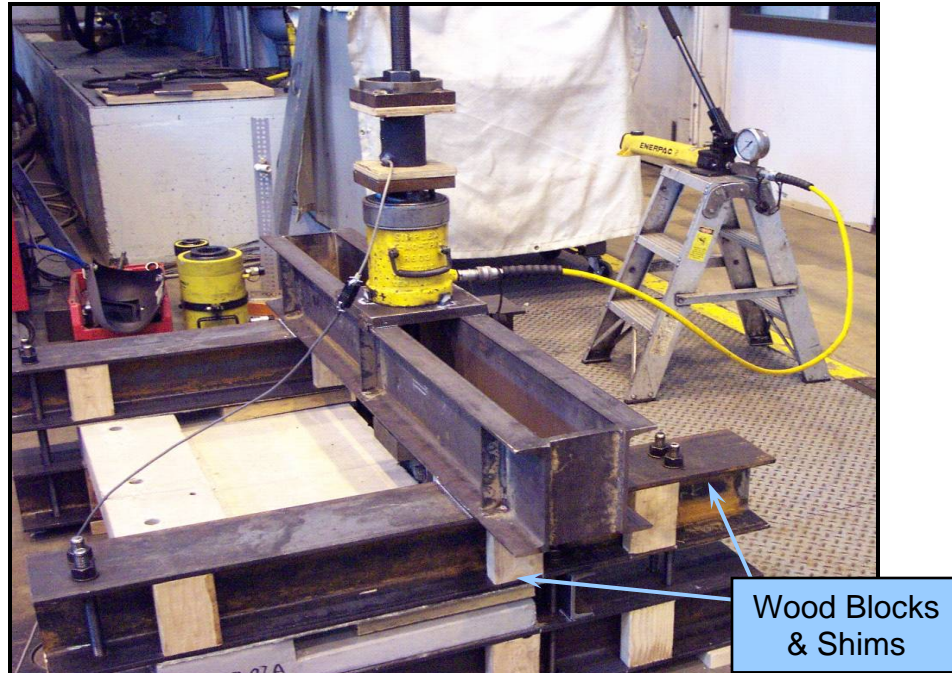
Figure 7-7. Side view of wood blocks and shims securing reduced thickness region
