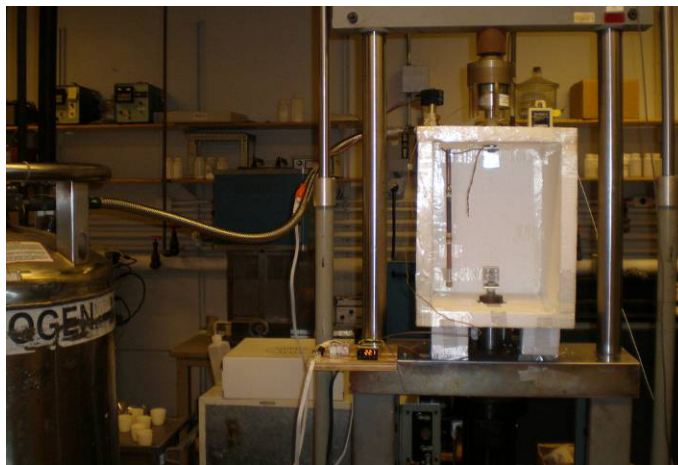
Figure 2.3 View of temperature-controlled test chamber
