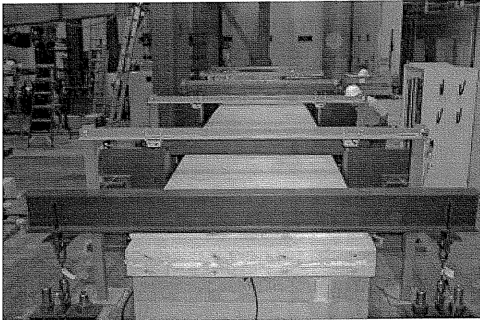
Figure 3.23 Steel frames used for mounting string pots.
