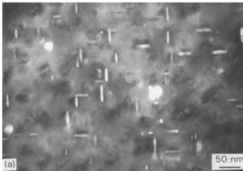
Figure 12. Dark-field micrograph of a CuNiSi alloy aged at 450°C for 750 hours with the beam direction parallel to the \langle 001 \rangle of the copper matrix using the (020)_{\text{ppt}} diffraction spot for imaging.[68]
