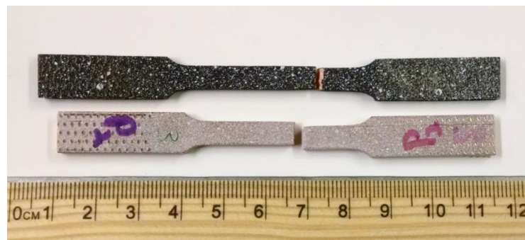
Figure 45. The two types of speckle patterns used for DIC strain mapping for (top) as-printed samples and (bottom) machined samples.
