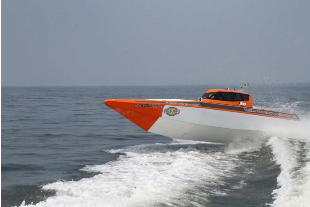
Figure 7-2: Numerette slamming test boat
