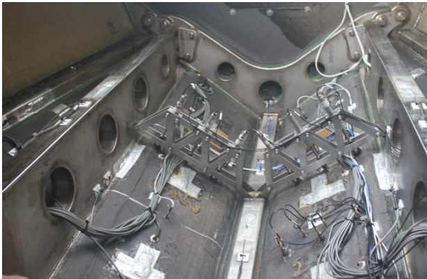
Figure 5-2: Port and starboard bottom panels, stainless steel longerons, bulkhead, and bottom sensors (pressure sensors, accelerometers, strain gages, LVDT's).
