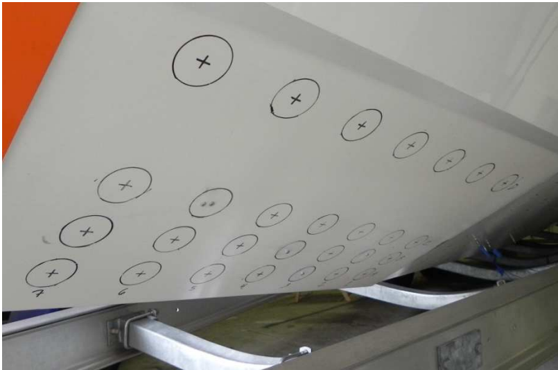
Figure 6-10 Static load test grid
