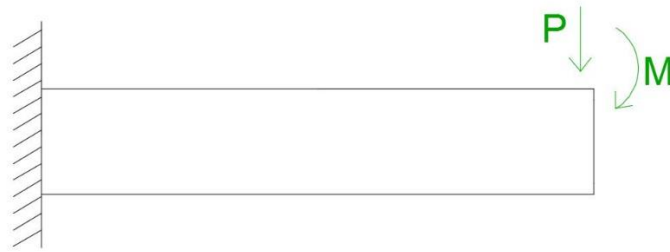
Figure 22: Reproduction of figure 4, Sketch representing the analyzed beam
