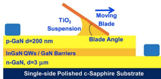
Figure 2-4: Schematic of rapid convective deposition of TiO 2 microspheres on top of InGaN LED samples [54].
