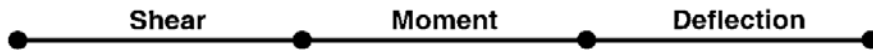
Figure A.17. Hypothetical series system model of typical girder (Estes and Frangopol 2001).
