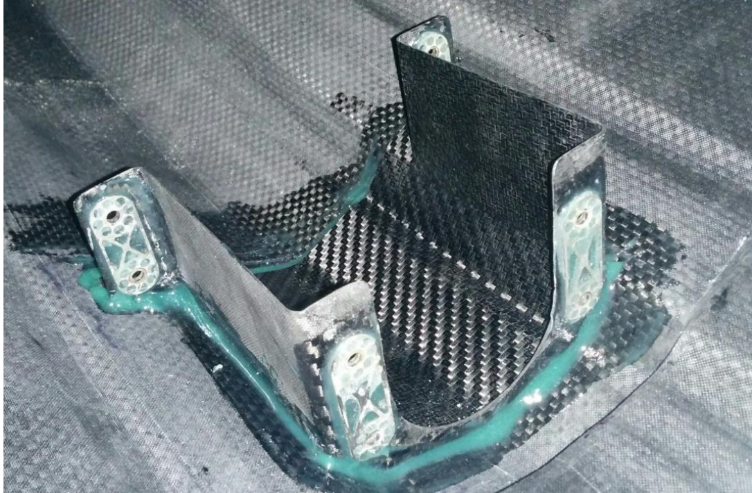
Figure 30: Bonded LORCA Motor Mount
