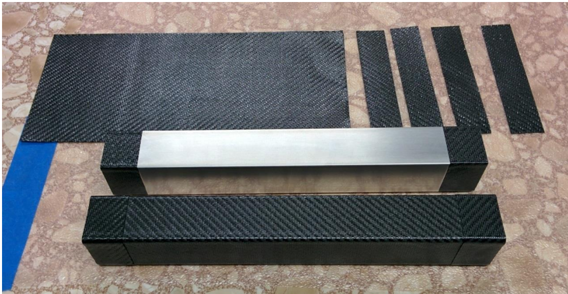
Figure 21: Laying Pre-Preg onto Battery Tray Molds
