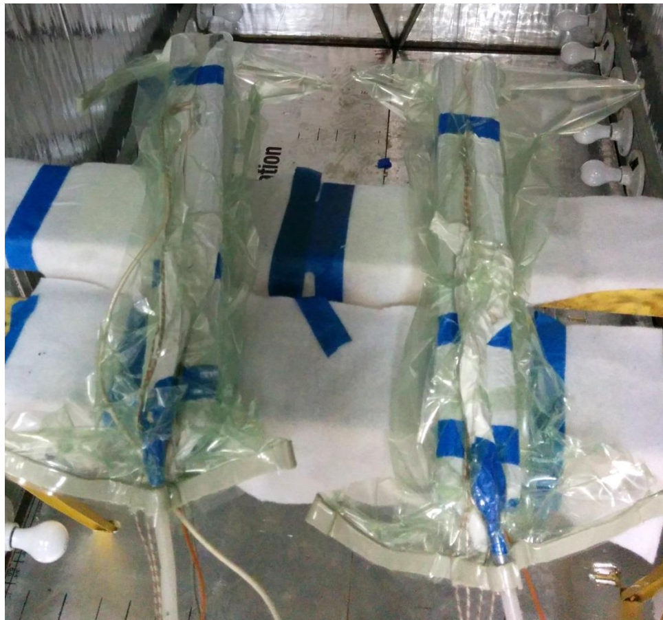
Figure 23: Two Molds Sitting under Vacuum
