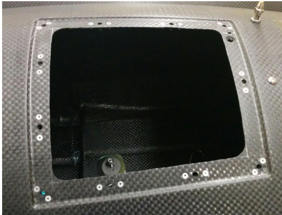
Figure 29: Access Hatch Lip
