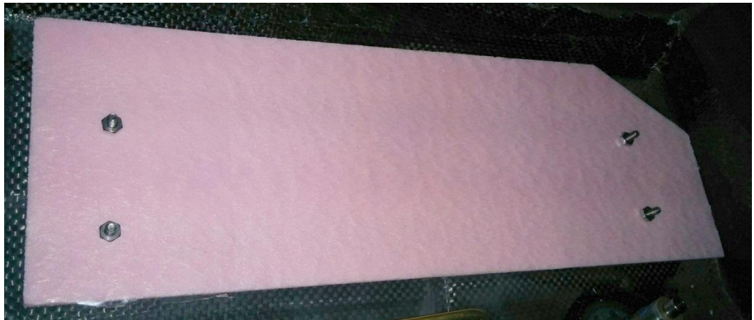
Figure 34: Bonding Mounting Studs for Battery Trays
