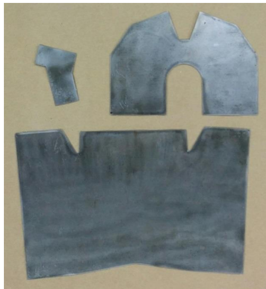
Figure 20: Motor Mount Ply Patterns
