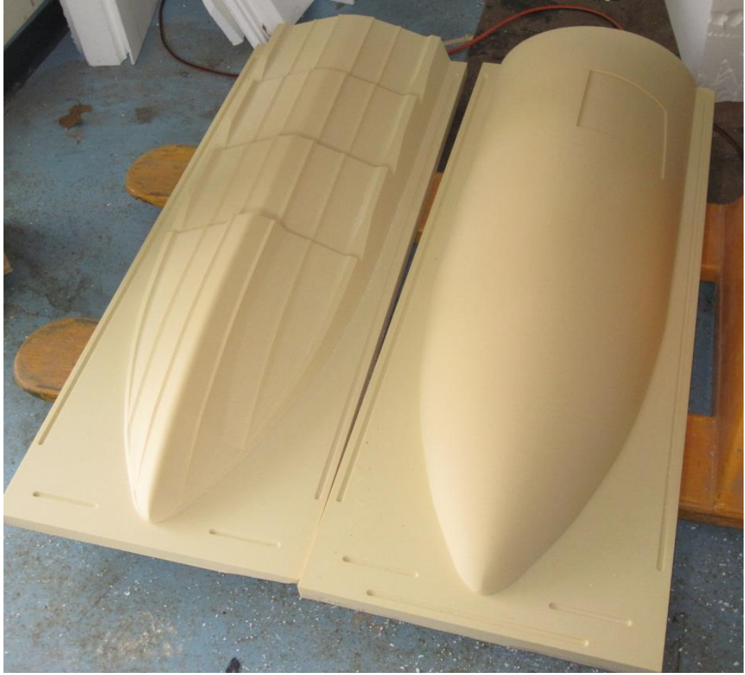
Figure 8: Completed LORCA Mold Plugs
