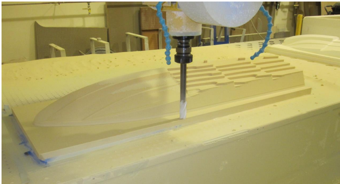
Figure 7: Machining LORCA Hull Plug
