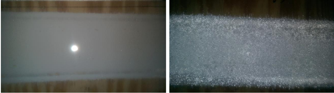
Figure 8: Epoxy roadway marking without glass beads (left) and with glass beads (right).
