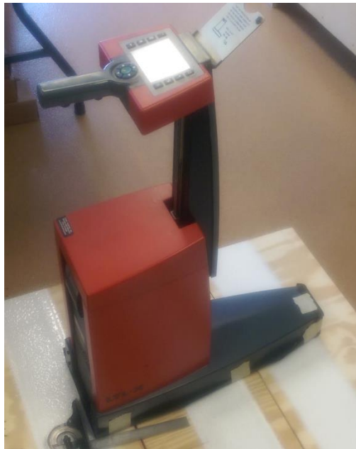
Figure 20: Modified Delta LTL-X handheld retroreflectometer.
