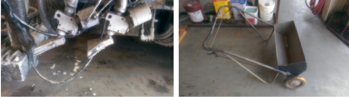
Figure 19: Bead gun applicator (left) and bead handcart applicator (right).
