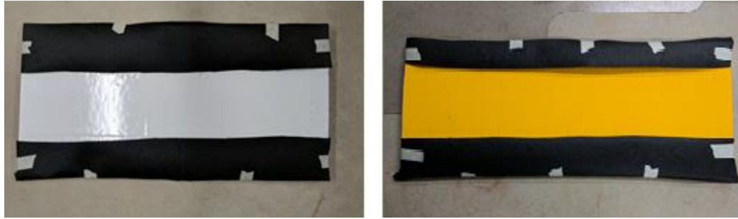
Figure 28: White (left) and yellow (right) roadway marking binder samples (without glass beads).
