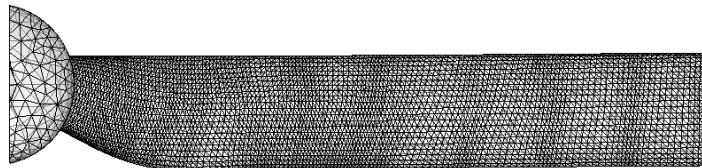
Figure 3.3: Finite Element mesh used for structural solver.
