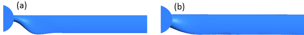
Figure 3.4: Blade shapes used for FSI analysis: (a) circular blade root, (b) parabolic blade root
