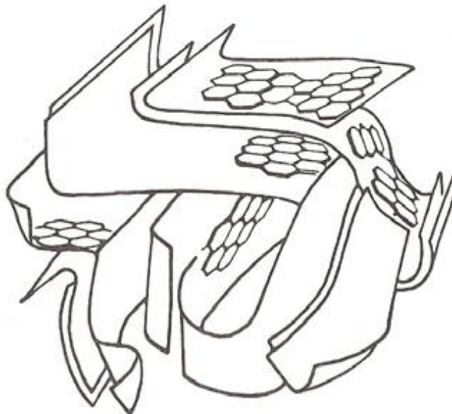
Figure 3.9. Schematic representation of the microstructure of activated carbons [146].
