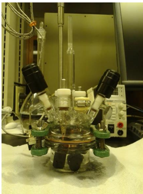
Figure 6.1. Custom made glass pressure cell used for SSA experiments.
