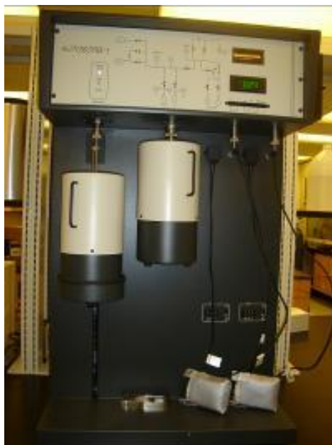
Figure 6.3. A photo of the Autosorb-1 instrument at Lehigh University available in Prof. Kai Landskron lab.
