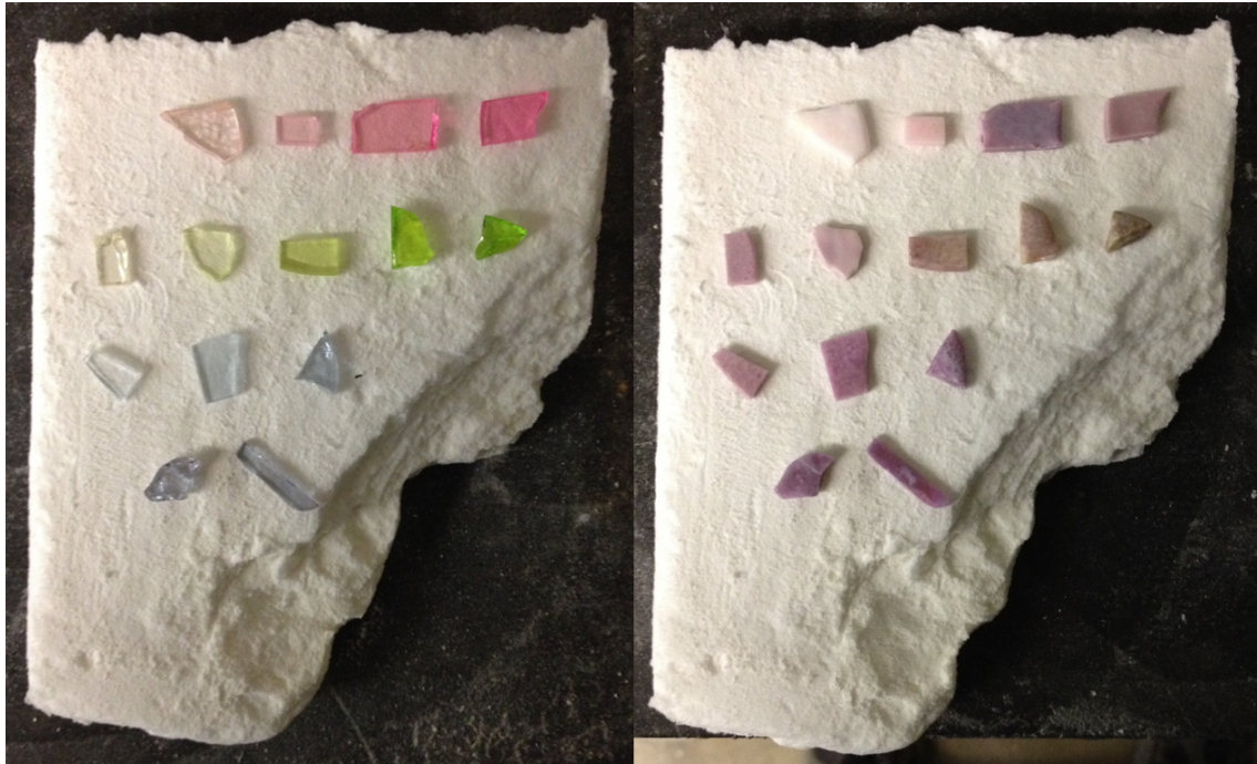
Figure 3.5: RE:LBGO glasses before (left) and after (right) furnace crystallization. Compositions (L to R): Row 1: Erbium, 1%, 4%, 10%, 20%, Row 2: Praseodymium, 0.2%, 1%, 4%, 10%, 20%, Row 3: Neodymium, 0.2%, 1%, 4%, Row 4: Neodymium, 10%, 20%
