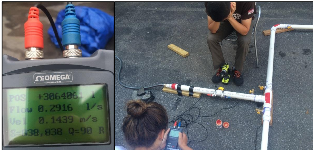
Figure 3.3: FDT-21 Ultrasonic Flowmeter: The flowmeter measures fluid velocity by the use of transducers that send and receive sound waves and measure transit time. Once velocity is found, the flowmeter calculates flow rate based on the inputted pipe diameter.
