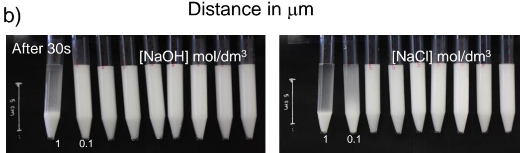
Figure 4.4 a) DLVO potential barrier for dilute suspension as a separation distance for different NaOH and NaCl concentrations, in mol/dm 3 — 10 -3 , — 10 -2 — 10 -1 — 1, b) sedimentation of 1% v/v suspension at different NaOH and NaCl concentration matching DLVO predictions.
