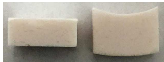
Figure 2: Left: line contact, Right: conformal contact
