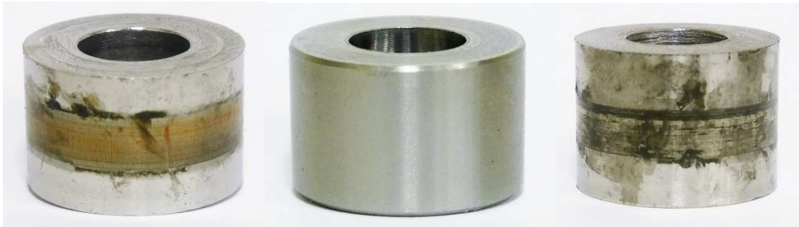
Figure 34: Left: ring after testing displaying orange film, Center: ring before testing, Right: ring after testing without orange film
