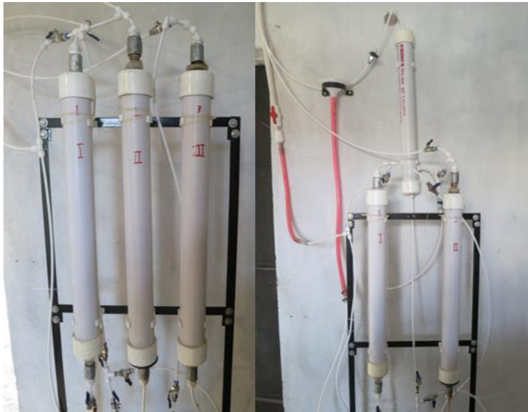
Figure 6.9. (L) Original construction design of three-column system; (R) Modified three-column system to include a decarbonator.
