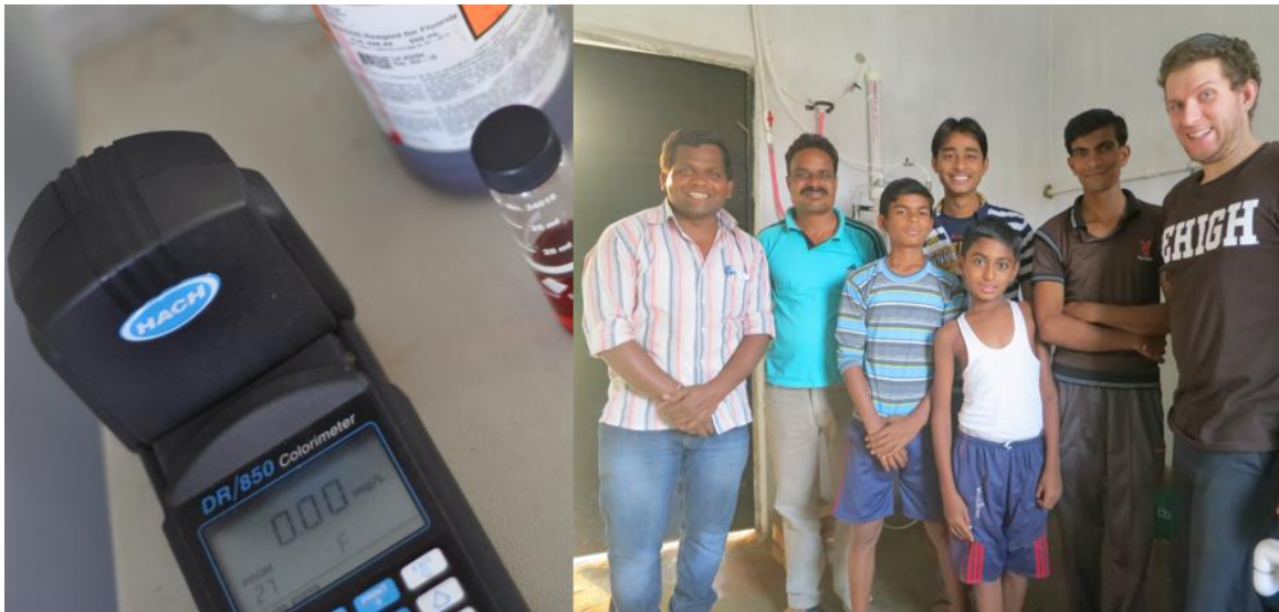
Figure 6.10. (L) HACH DR/850 used for fluoride testing along with SPADNS solution; (R) group photo of Rite Water installers, local community observers, and myself.
