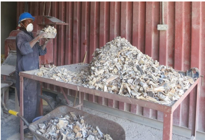
Figure 11.2. A worker sorting bones before grinding and crushing them into smaller pieces.
