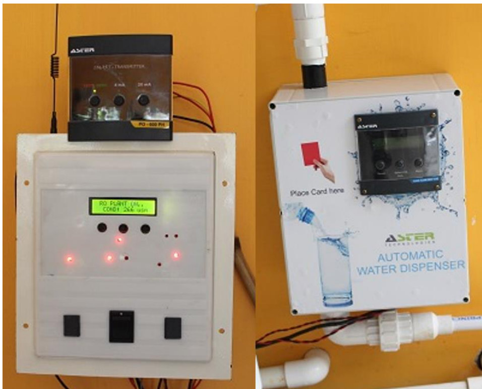
Figure 3.14. Water ATM installed in Baduria for automatic, metered water dispensing without requiring the presence of a caretaker.
