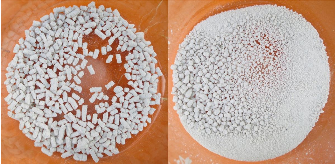
Figure 4.2. Fresh HAP in a beaker (L). HAP crumbles after finger pressure (R).
