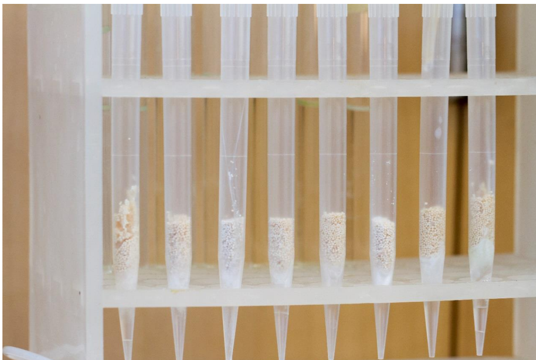
Figure 3.1. Mini-column setup for HAIX-NanoZr used for capacity testing under different pH values. Created by Jinze Li.
