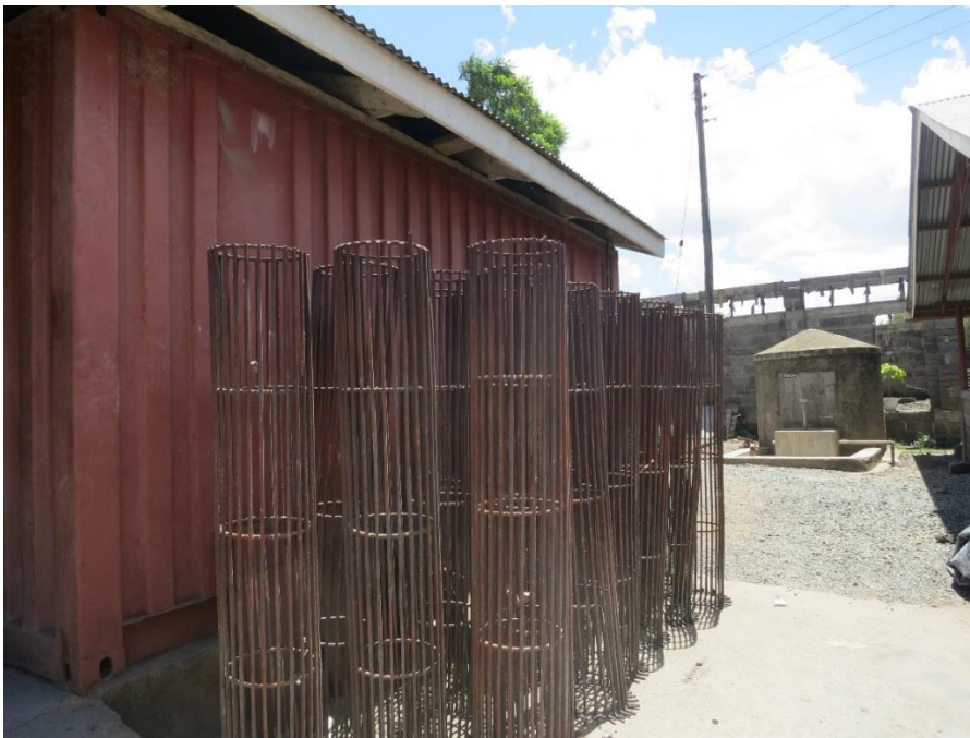
Figure 11.4. Steel tubes used for spacing the bones inside the furnace for more uniform air flow.
