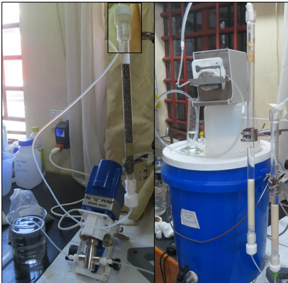
Figure 3.6. Original FMI pump attached to a single column with sealed fittings (L). The gravity-driven system and peristaltic pump- open to the atmosphere, with columns at different elevations (R).
