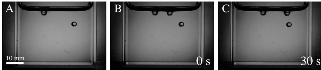
Figure 6.2: (A) Figure illustrating fine balances of the elastic, wetting and gravitational forces giving rise to different types of stabilities of glass spheres (3.2 mm diameter) released on the surface of a polyacrylamide hydrogel of modulus 10 Pa. An untreated (hydrophilic) glass sphere (right) immediately plunges into the gel and becomes neutrally buoyant afterwards. A hydrophobic glass (left) floats on the surface of the same gel. (B) This is an extension of the experiment in A, that shows when another hydrophobic particle is released in between the two, (C) it gets strongly attracted toward the hydrophilic particle, but moves on the gel's surface to minimize its distance of separation from the latter.
