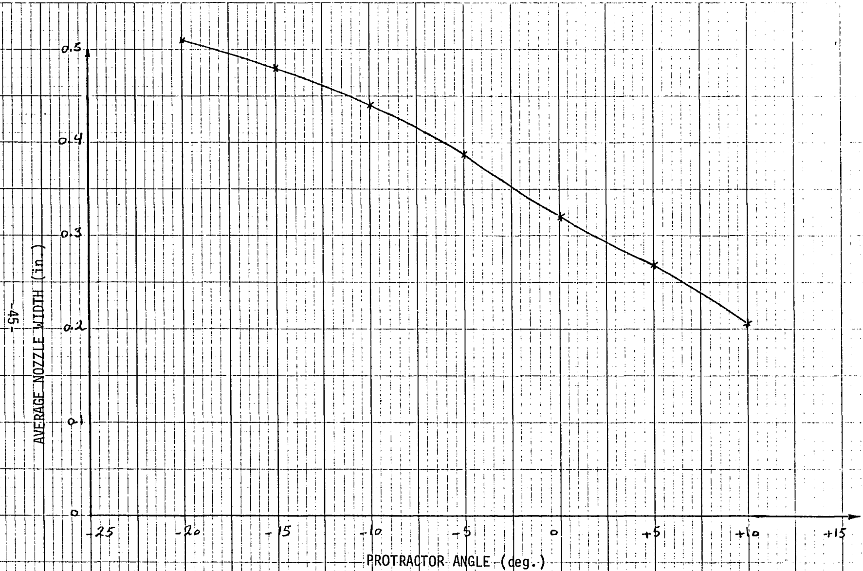
FIG. 11 Average measured throat width versus protractor angle reading.
