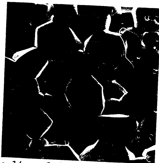
Figure 14a. 1.0 \mu\text{m} \leftarrow Scanning electron micrograph of polished and acid-etched sample with Sr/Ti = 1.000, slow-cooled from 1400°C.
