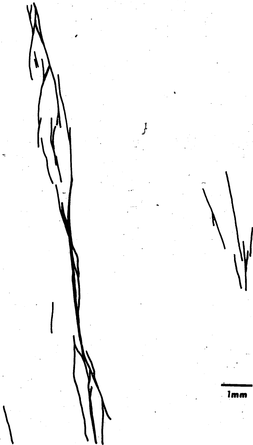
Figure 12 : Tracing of Foliation from Thin Section of Sample 79-31.
