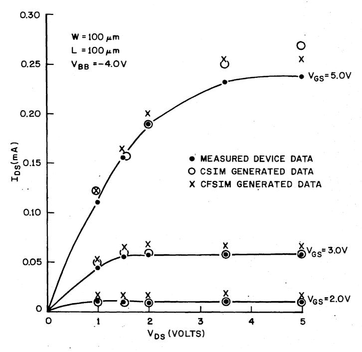
DRAIN-CURRENT CHARACTERISTICS FOR A WIDE, LONG CHANNEL TRANSISTOR
