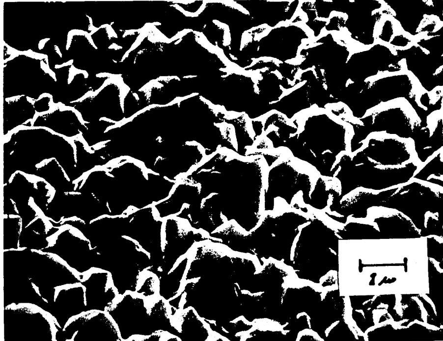
FIG. 14 Au DEPOSITED AT 9% DUTY CYCLE: 0.1 msec ON, 1 msec OFF; 10,000X
