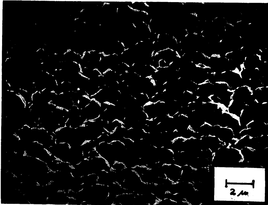
FIG. 38 Au DEPOSITED AT 66% DUTY CYCLE: 2 msec ON, 1 msec OFF; 5,000X
