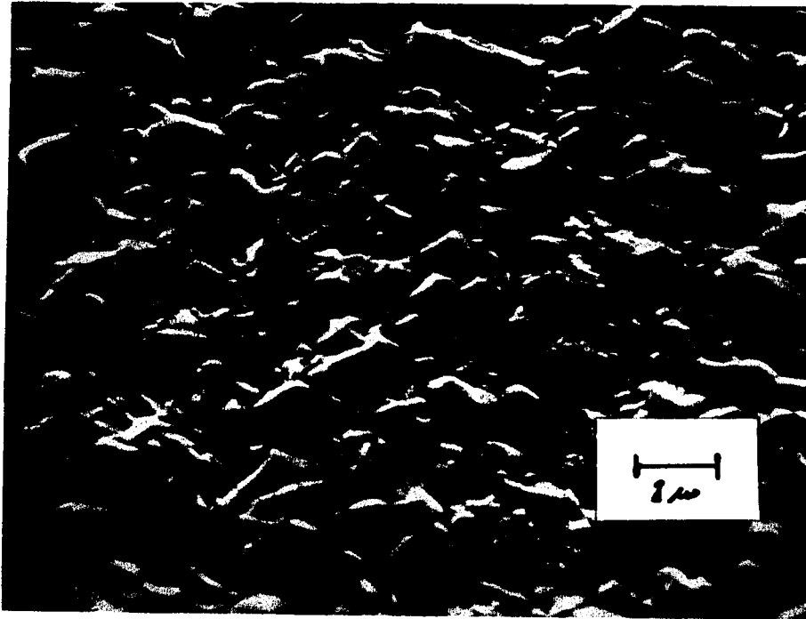
FIG. 20 Au DEPOSITED AT 9% DUTY CYCLE: 6.0 msec ON, 60 msec OFF; 10,000X
