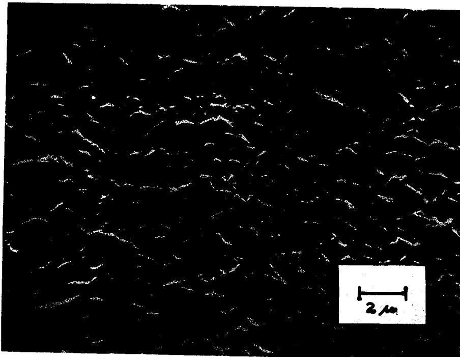
FIG. 33 Au DEPOSITED AT 33% DUTY CYCLE: 4.0 msec ON, 8 msec OFF; 5,000X
