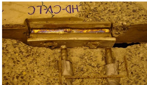
Figure 4.42. Damage state at 1.60-in shear opening
