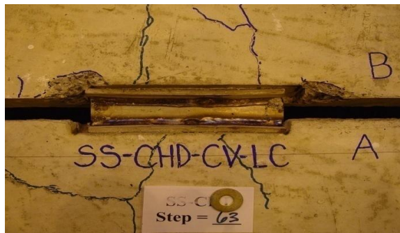
Figure 4.41. Damage state at 0.80-in shear opening
