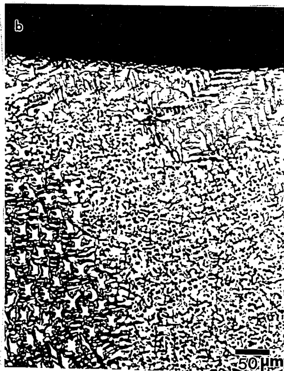
Figure 27. As-welded microstructure of the 316L SS weld overlay coating; (a) top of the coating; (b) delta ferrite in austenitic matrix. Etchant: electrolytic-5V [60% HNO 3 and 40% water] solution.
