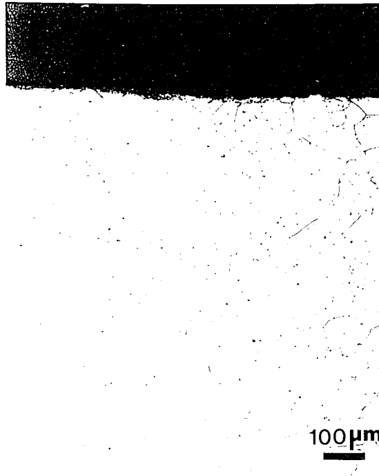
Figure 27c. Microstructure of the wrought 316L SS alloy. Microstructure consists of austenite grains and annealing twins.
