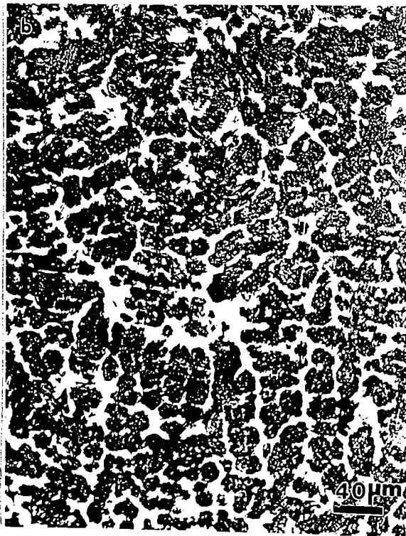
Figure 28. As-welded microstructure of the 420 SS weld overlay coating; (a) top of the coating; (b) dendrites of the lath martensite. Etchant: Viella reagent.
