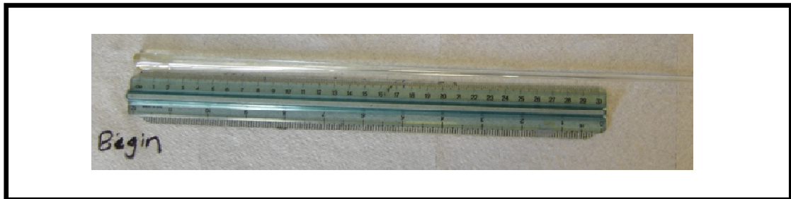
Figure 4.11 Tube preform extruded at 358°C
