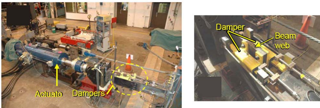
b. Photo of Physical Substructure Setup
