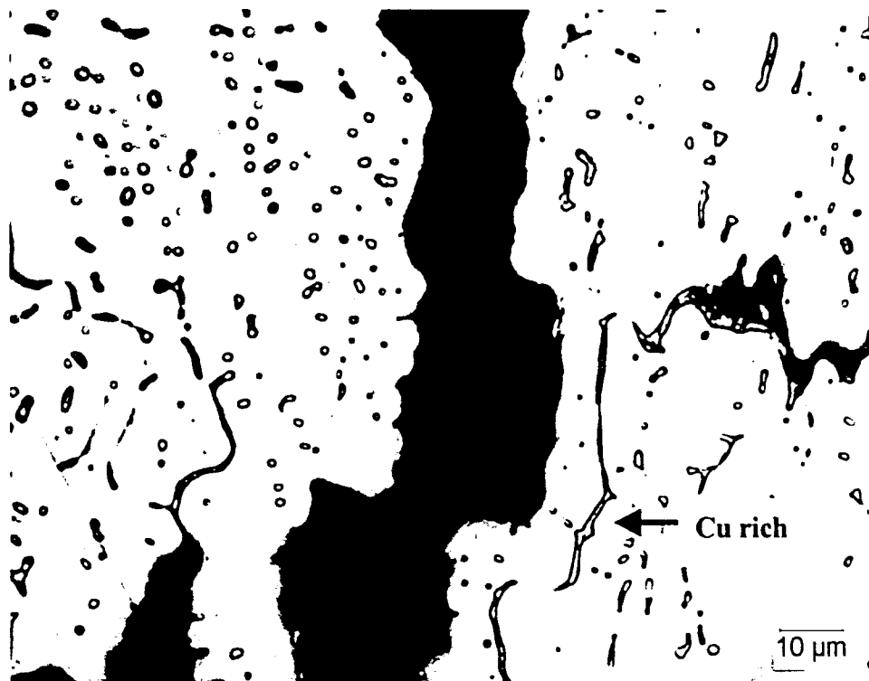
Figure 22: Fe-13.2Ni-15.5Cu. Cracking along Cu rich regions. Increased Ni results in less terminal Cu compared to Figure 21.
