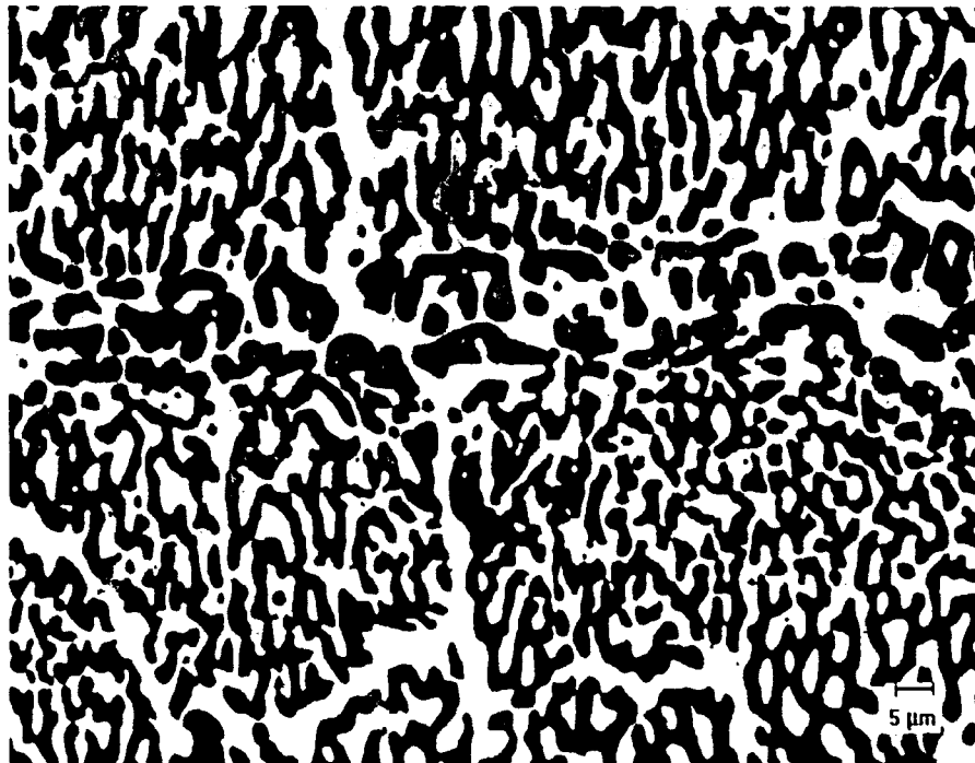
Figure 7 a and b: Steel - 51.6 wt% Cu. Fully interpenetrating Fe rich (dark) and Cu rich (light) networks in liquid phase spinodal structure that is crack free
