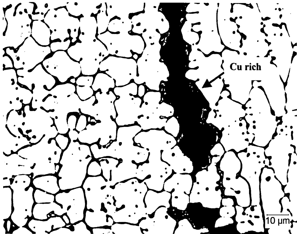
Figure 21: Fe-2.5Ni-17.0 Cu. Cracking observed along Cu rich regions.
