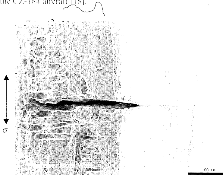
Figure 2.8: SEM micrograph of corrosion-related distributed damage at hole #54 in panel B2-2-2 of the CZ-184 aircraft [18].
