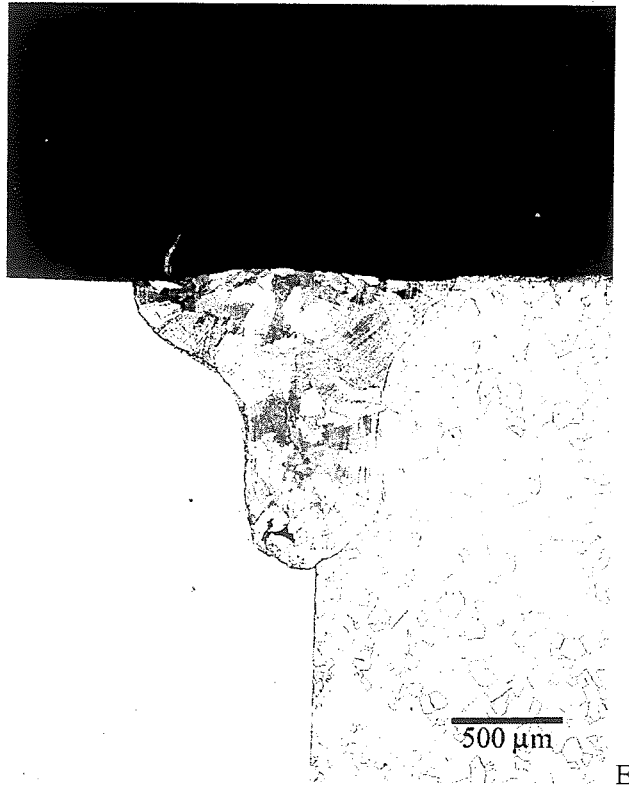
Figure 5.6 – E) Micrograph of dissimilar metal laser welds illustrated effect of changing beam position relative to base metal interface. Laser at materials interface, B2 is on the left.
