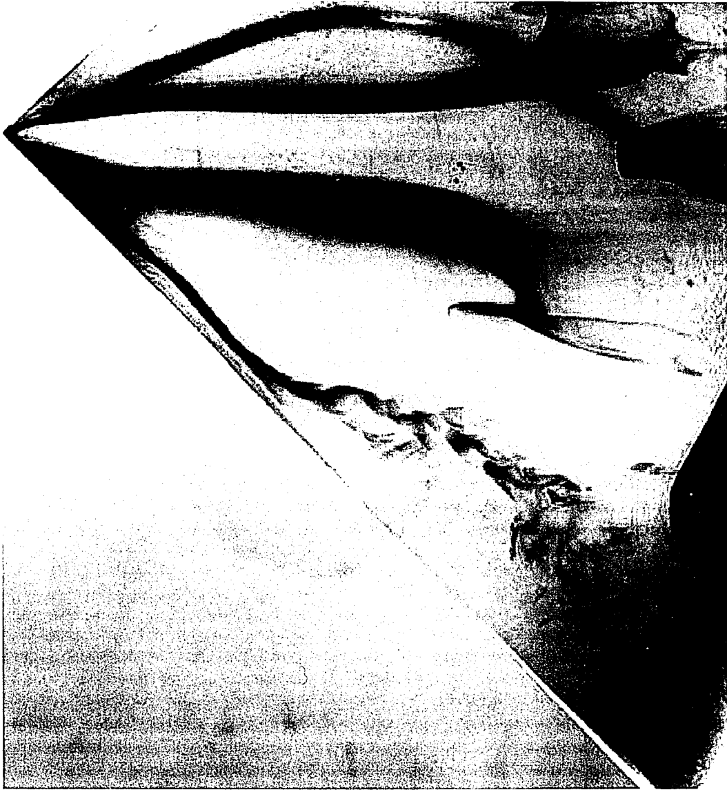
Figure 1.1: Dye visualization of flow structure at angle-of-attack \alpha = 12^\circ and for a value of Reynolds number Re = 32,000 based on chord (Ol, 2006).
