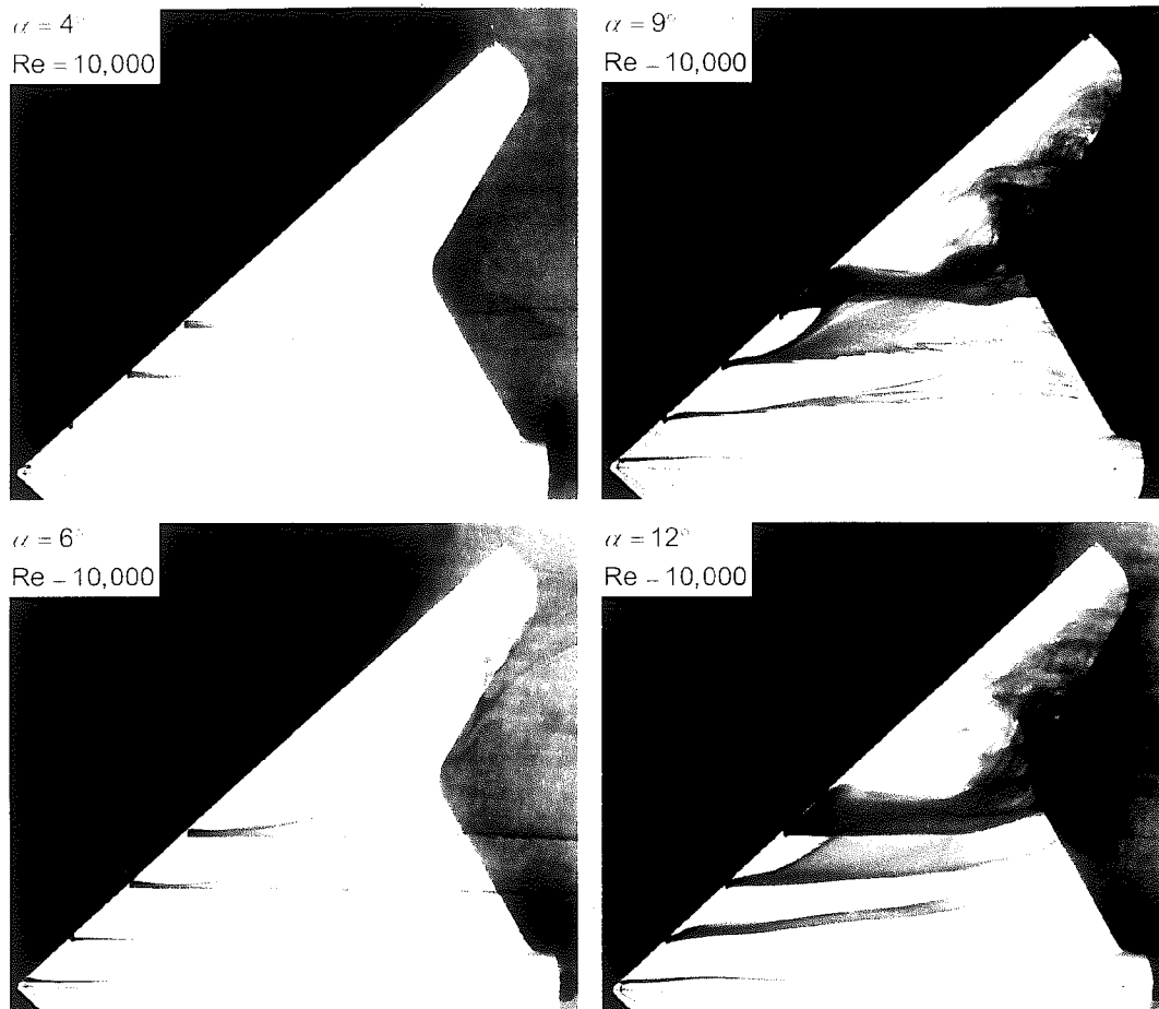
Figure 3.3: Dye visualization of flow structure for angles of attack \alpha = 4^\circ, 6^\circ, 9^\circ and 12^\circ at a value of Reynolds number Re = 10,000 based on chord
