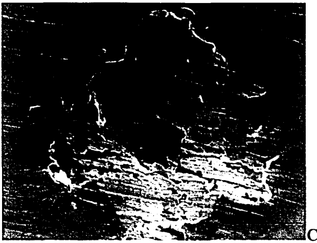
Fig. 4-20 A and B) Pits in AL-6XN base metal occurring at 70°C and C) a higher magnification of the pit seen in B) showing evidence of undercutting.
