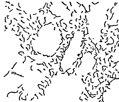
Type D Inter-Dendritic Segregation, Random Orientation.
