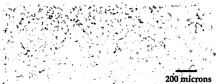
Figure 22b. Cross-sectional light optical micrograph of decarburized sample after grinding and polishing operations. The depth of the decarburization is 400 \mu m (50x)
