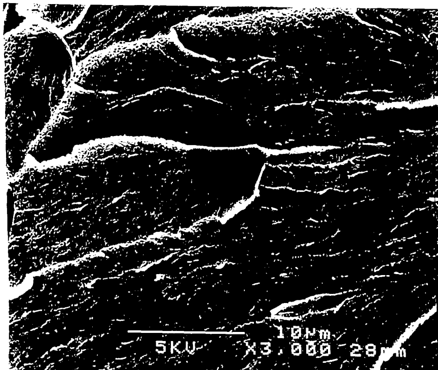
Fig. 4-9 SEM micrograph taken from the stress-whitened zone of the model system(model 1). As seen in this figure, the interfaces between epoxy particles and epoxy matrix do not interfere with the crack propagation.
