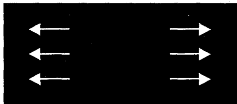
Figure 2- 2. Schematic illustration of 2-D heat flow conditions that exists when the plate thickness is on the same order as the weld depth.
