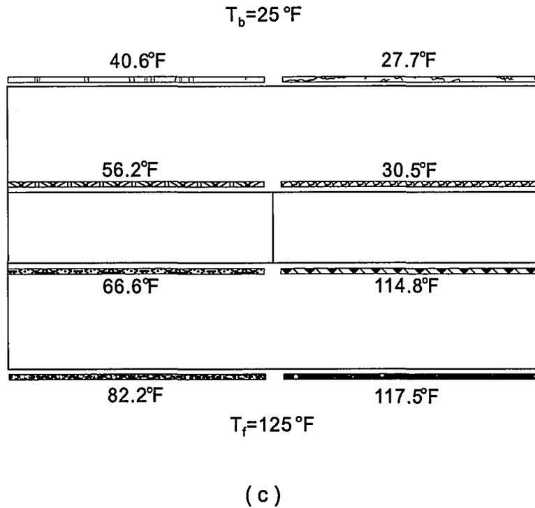
Figure 3.3 Summary of parallel flow calculations results: (a) thermal resistance; (b) heat flux; (c) temperature distribution.
