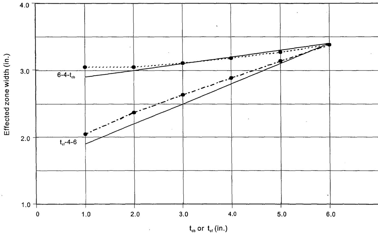
Figure 4.11 Variation in  $E_z$  with concrete wythe thickness for unsymmetric characteristic sections.
