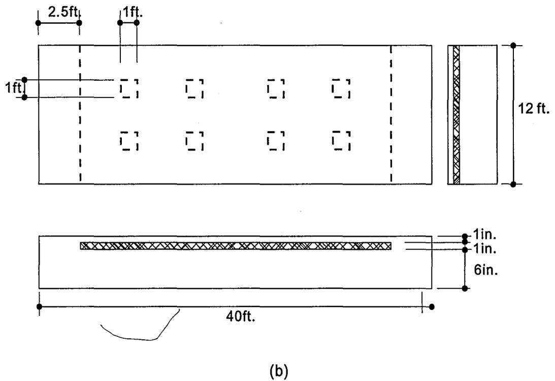
Figure 4.15 Typical precast concrete sandwich wall panels which are unsymmetric through the thickness:(a) 1-1-6 panel; (b) 6-1-1 panel.
