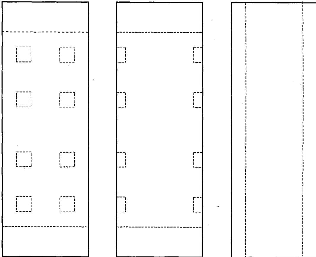
Figure 2.1 Three typical configurations of precast concrete sandwich wall panels.
