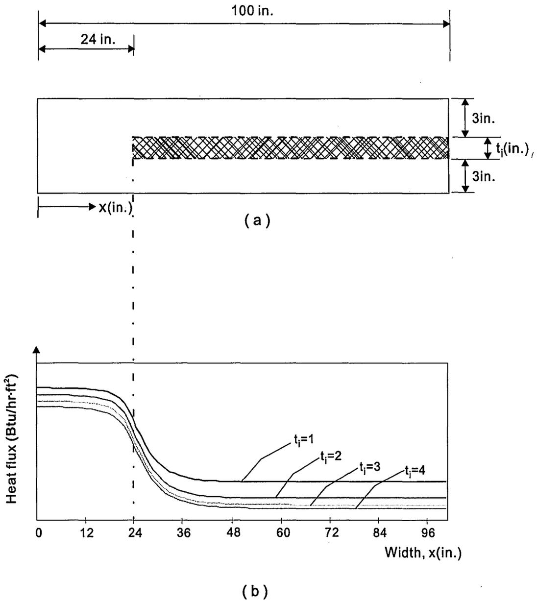
Figure 4.5 Effect of insulation thickness: (a) characteristic section; (b) heat flux along the width of the panel.
