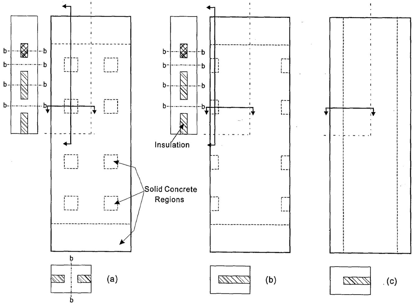
Figure 4.2 Defining a characteristic section from three typical precast concrete sandwich wall panels.
