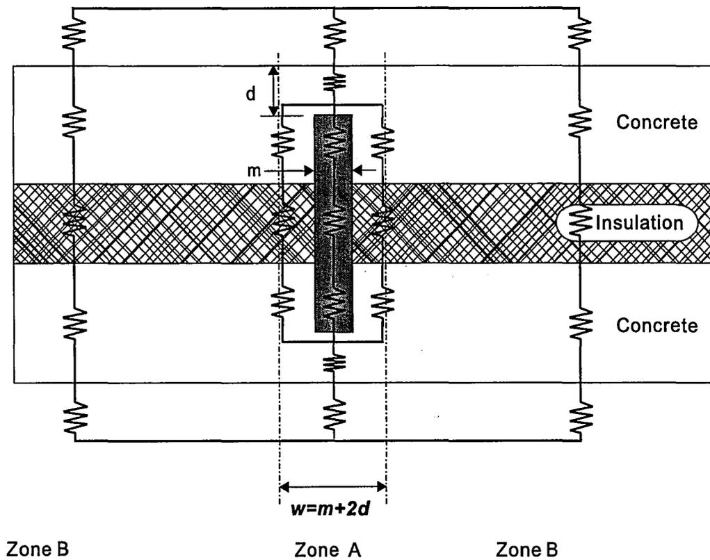
Figure 2.6 The electric circuit based on the zone method.
