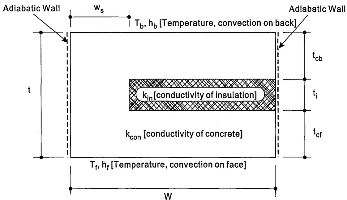
Figure 4.4 Description of notation for the characteristic section.
