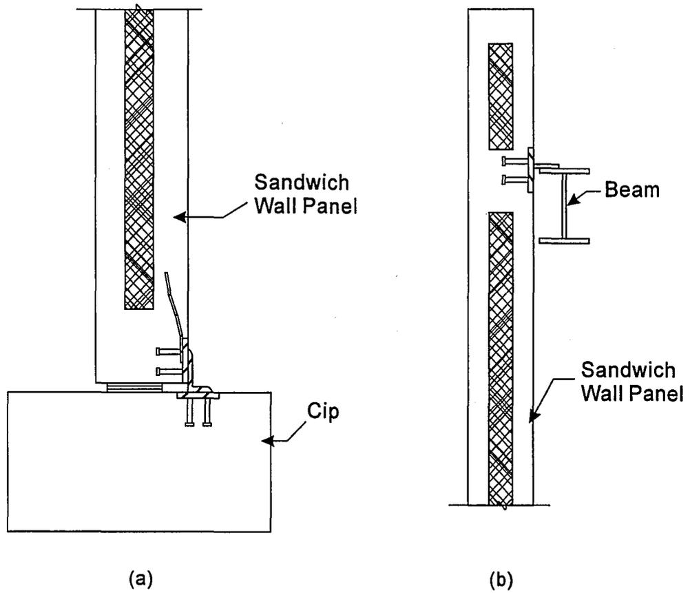
Figure 2.2 Example solid concrete connection regions: (a) connection between the vertical wall and foundation; (b) connection between vertical wall and horizontal span.
