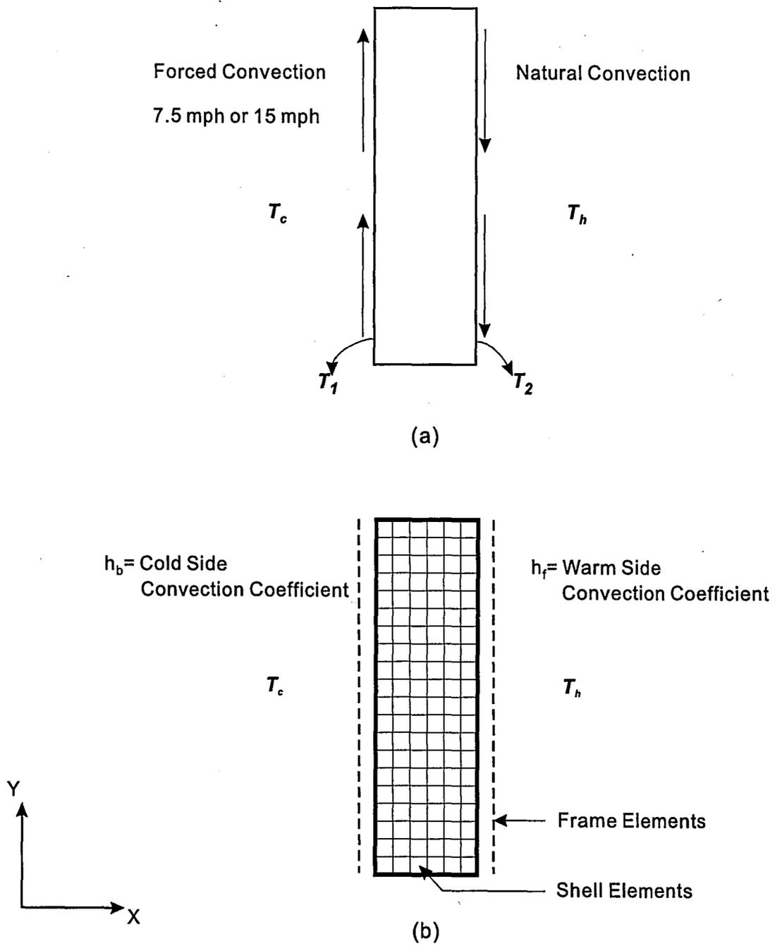
Figure 2.9 Finite element modeling of guarded hot box test (2D): (a) actual test assembly; (b) finite element model.
