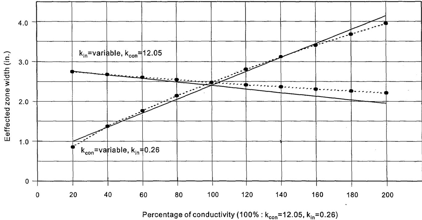
Figure 4.12 Variation in  $E_z$  with concrete and insulation thermal conductivities for a 3-2-3-24 characteristic section.
