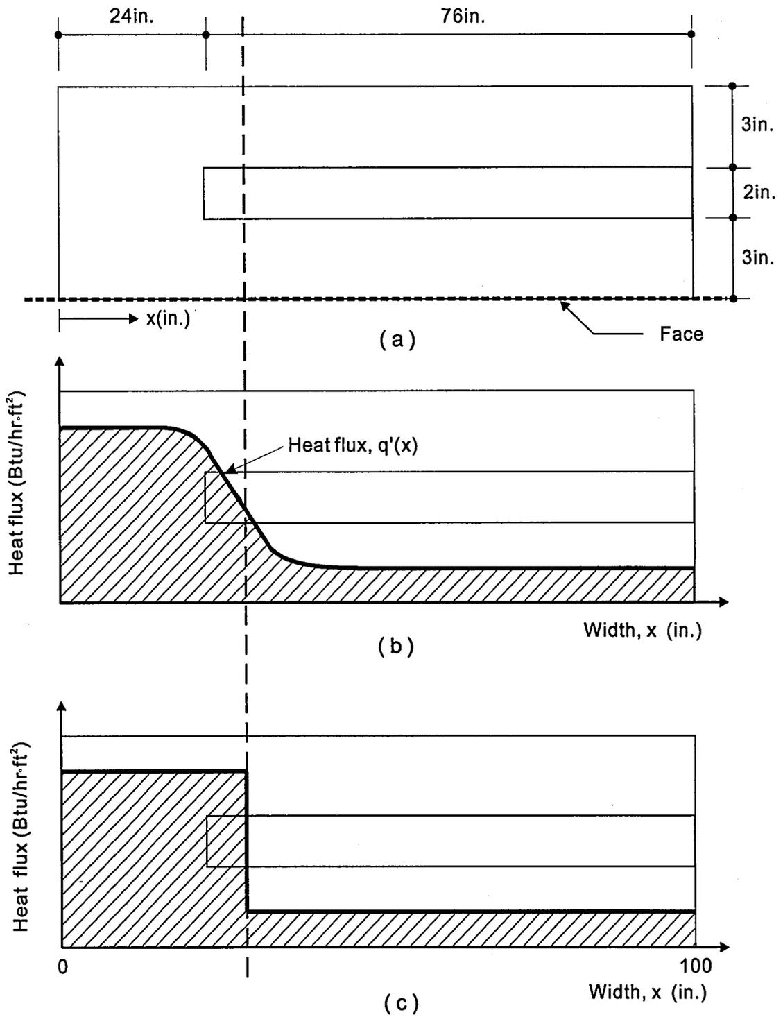
Figure 4.8 Heat flux trough characteristic section: (a) specified characteristic section; (b) heat transfer rate along the face of the characteristic section; (c) simplified representation of heat flux.
