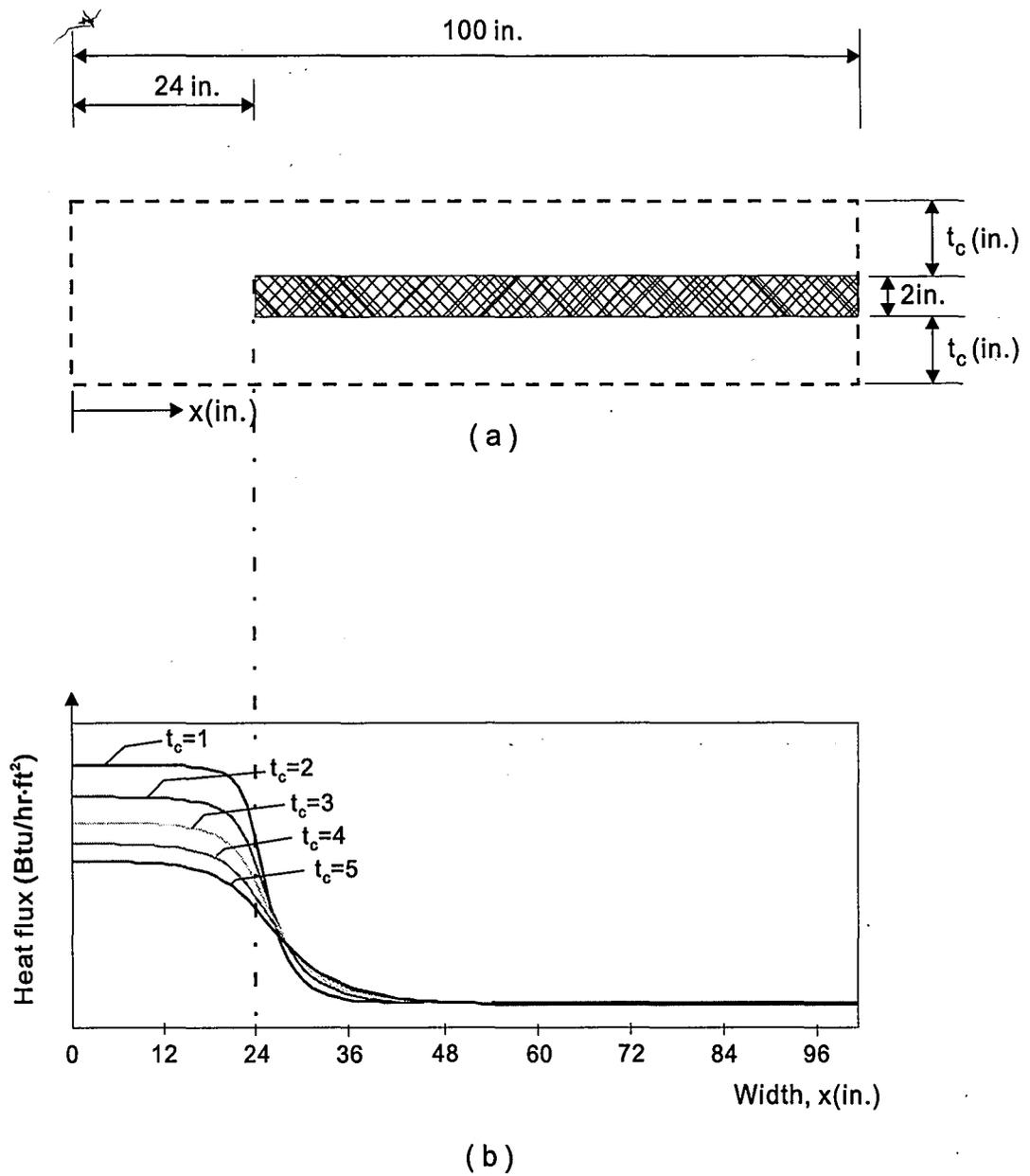
Figure 4.6 Effect of concrete thickness: (a) characteristic section; (b) heat flux along the width of the panel.
