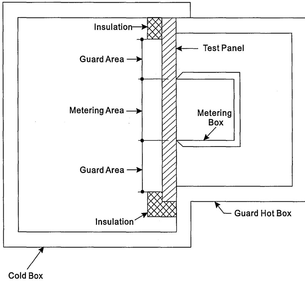
Figure 2.7 Schematic arrangement of the major components of the guarded hot box system (ASTM C236).
