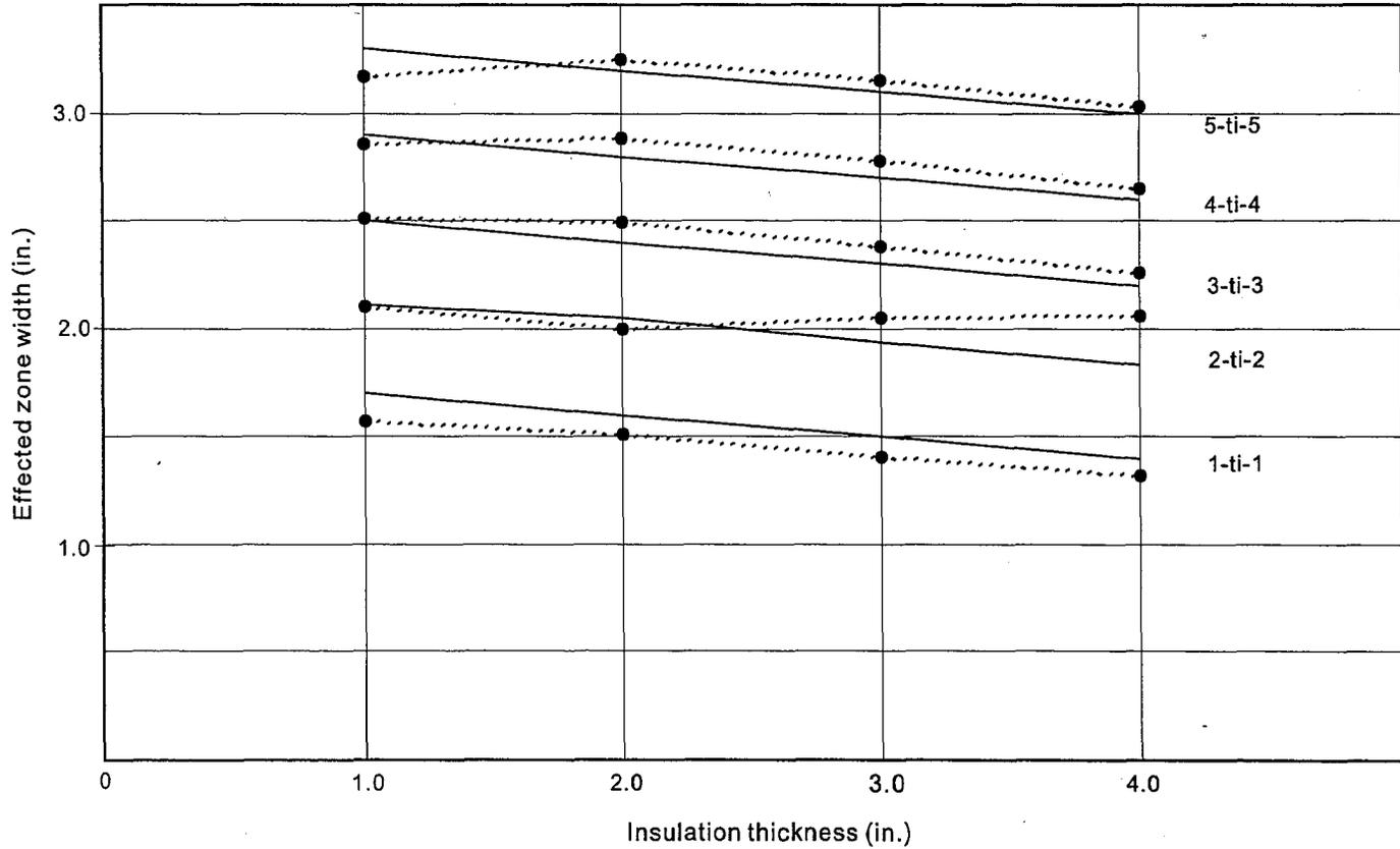
Figure 4.10 Variation in  $E_z$  with concrete wythe thickness and insulation layer thickness for symmetric characteristic sections.
