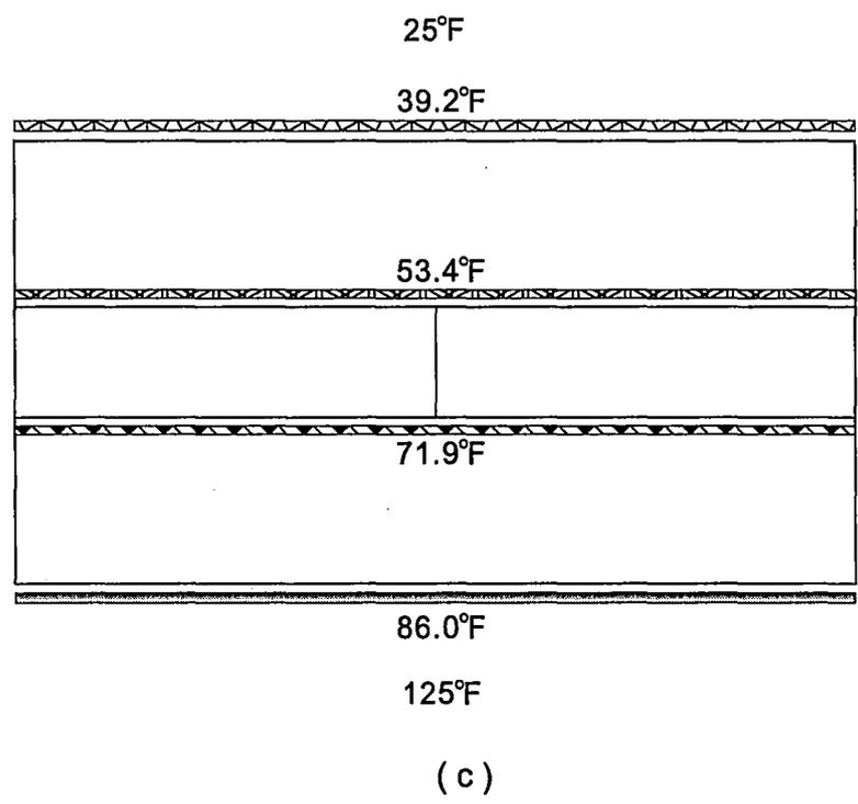
Figure 3.5 Summary of results of isothermal plane calculations: (a) thermal resistance; (b) heat flux; (c) temperature distribution.
