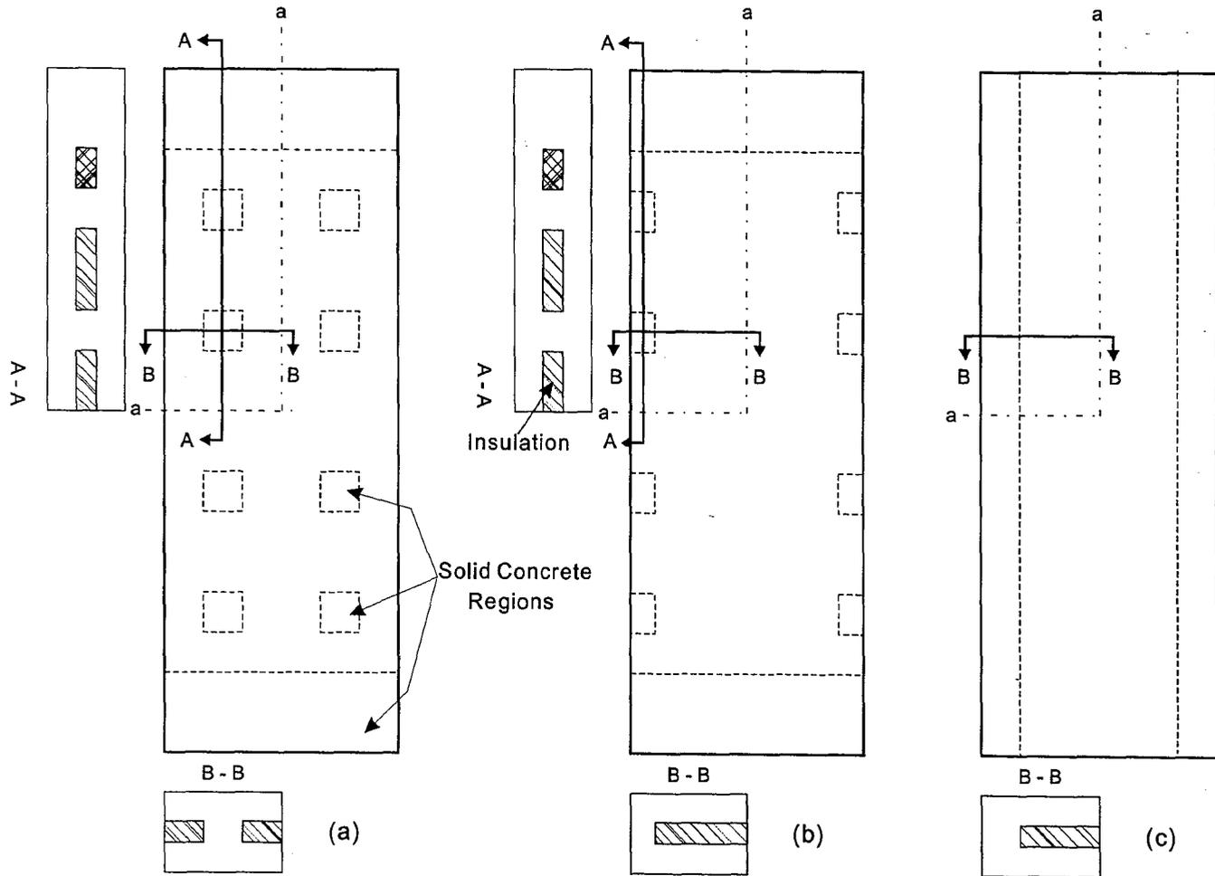
Figure 4.1 Three typical precast concrete sandwich wall panels with sections a-a that show quarter symmetry of each panel.
