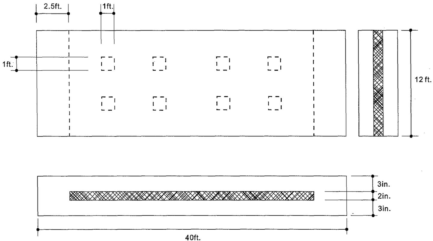
Figure 4.13 Typical precast concrete sandwich wall panels which is symmetric through its thickness.
