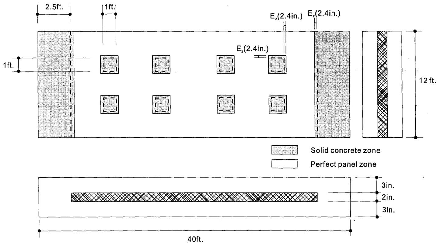
Figure 4.14 Typical precast concrete sandwich wall panel (same panel as Figure 4.14) showing solid concrete zones increased by  $E_z$ .
