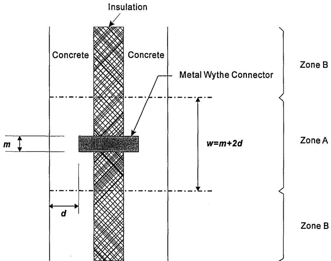
Figure 2.5 The determination of the width of the zone based on the zone method.
