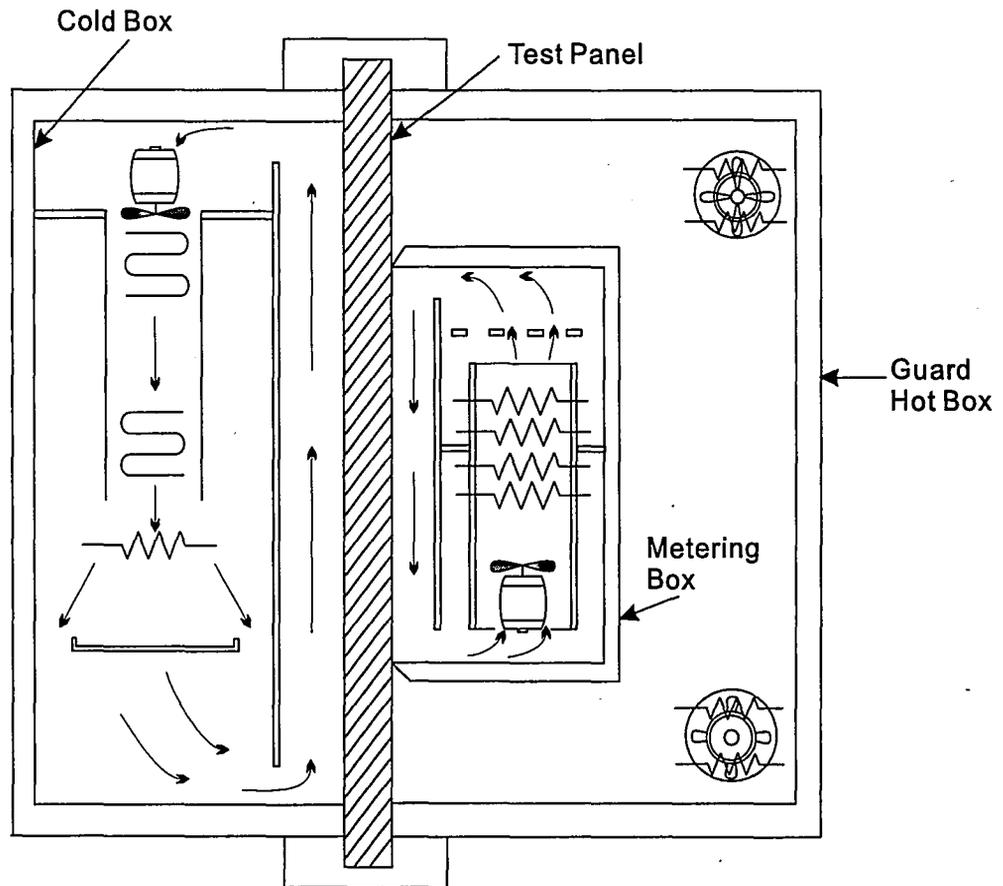
Figure 2.8 Detailed arrangement of equipment in guarded hot box test (ASTM C236).
