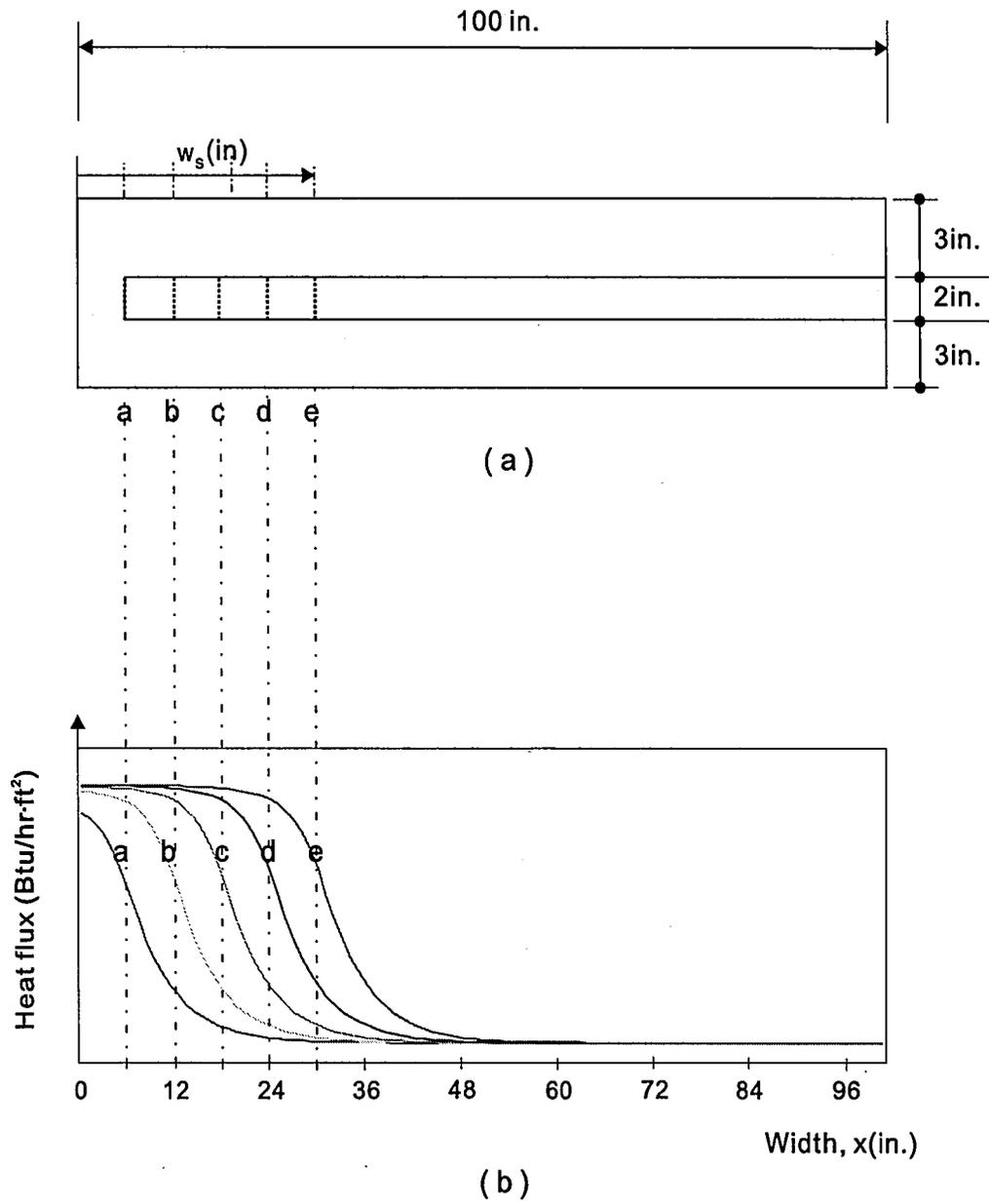
Figure 4.7 Effect of solid concrete width: (a) characteristic section; (b) heat flux along the width of the panel.
