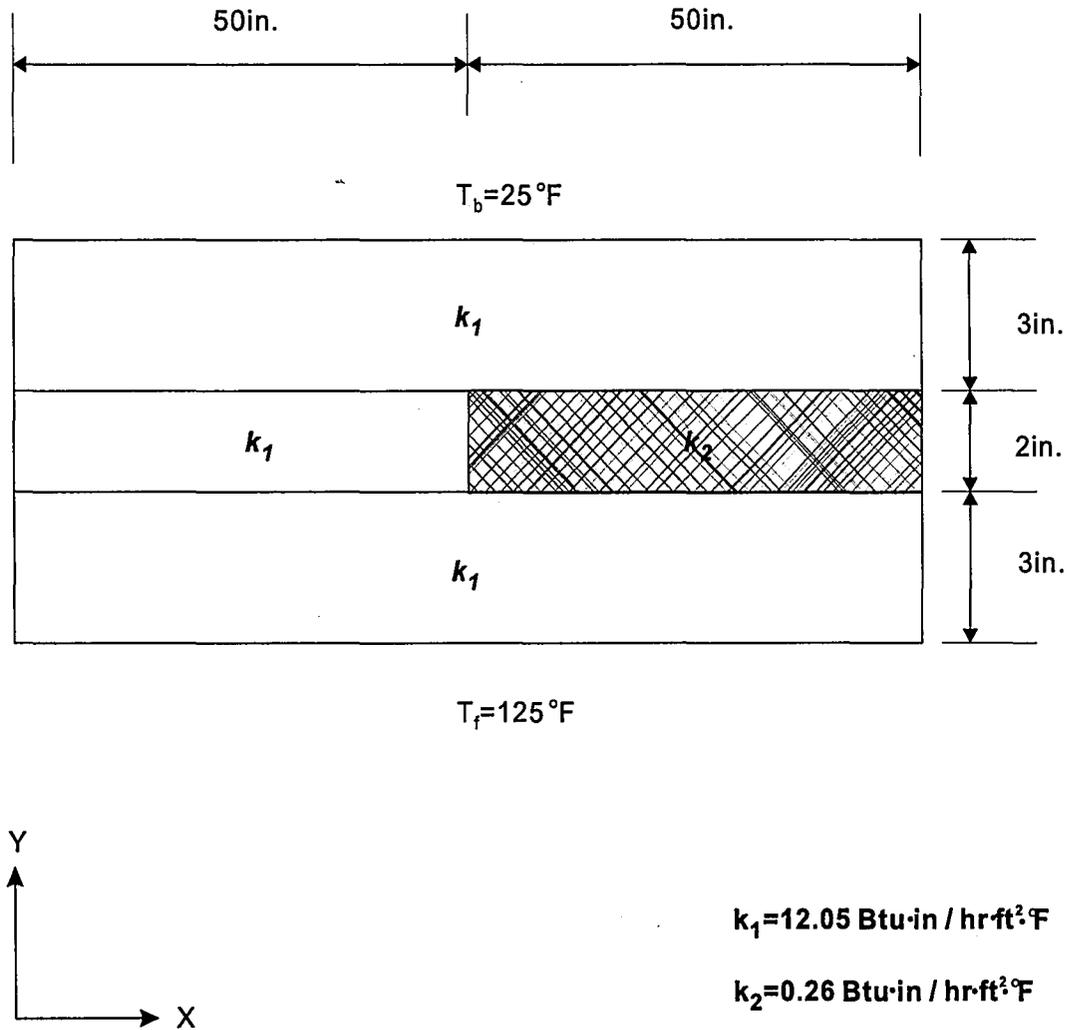
Figure 3.1 Example assemblage of materials used to compare classical calculation methods and finite element method.
