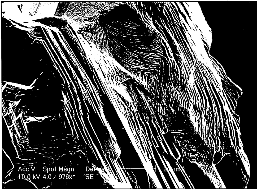
Figure 4: Morphology and scale of fine-scale structure present on fractured surfaces of CBN abrasive particles.
