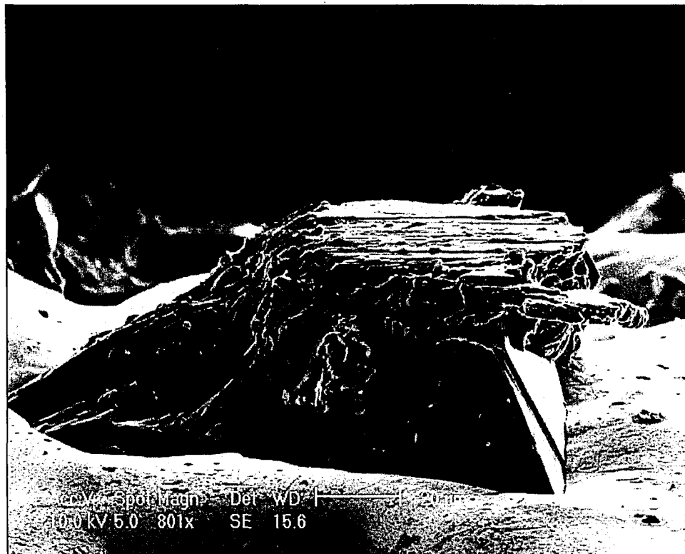
Figure 69: Encapsulation of a single CBN grain by adhering material.
