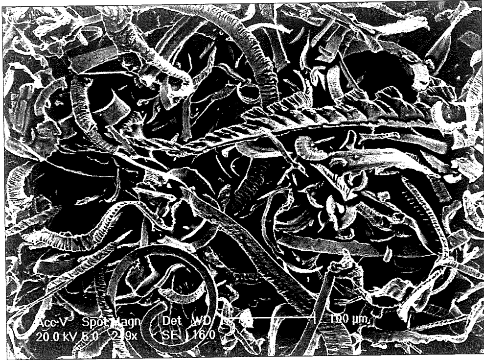
Figure 64: Collection of grinding chips with various shapes and sizes.
