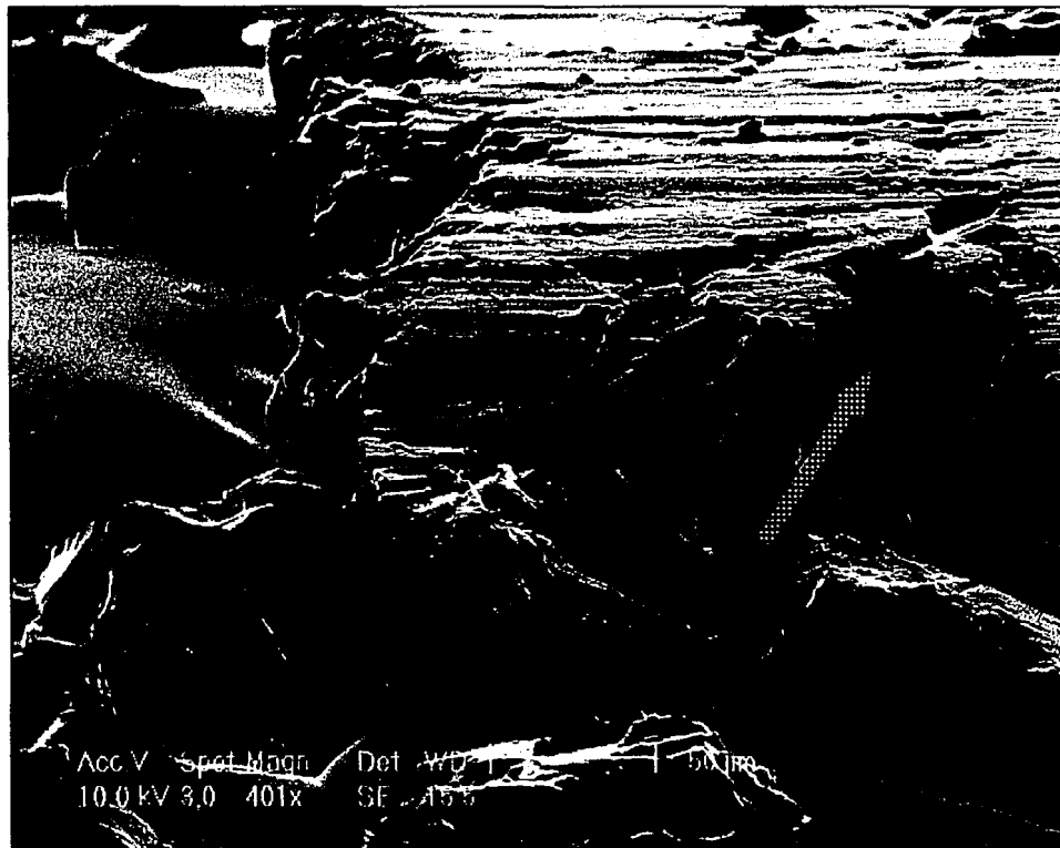
Figure 77: Build-up at the rake face showing the direction of material flow.
