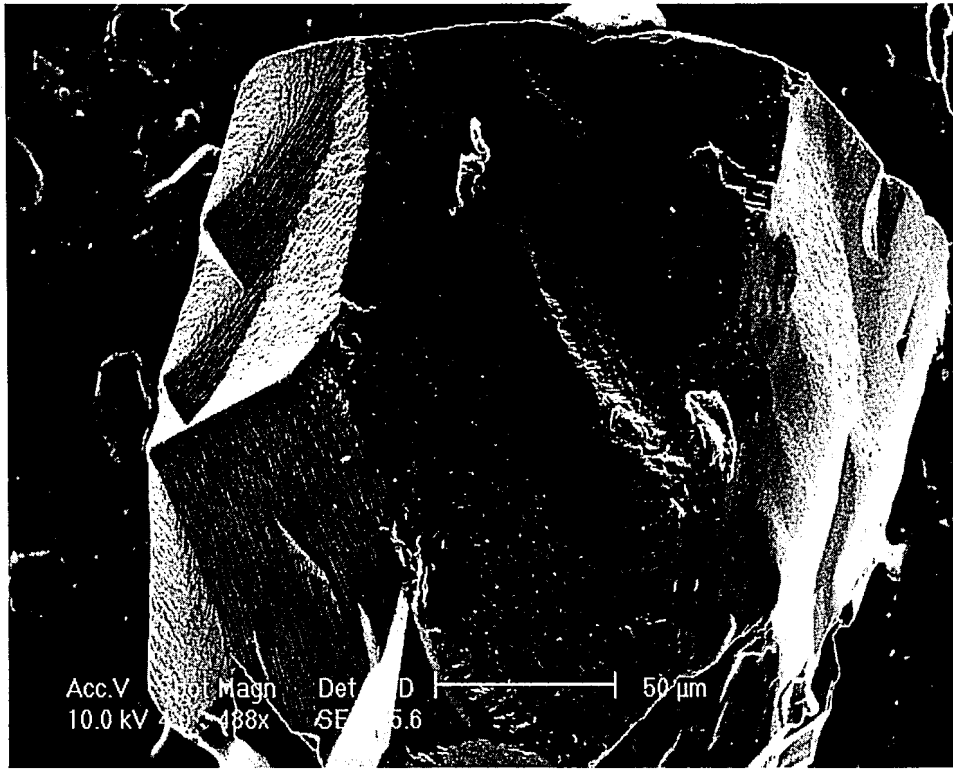
Figure 90: CBN control grain with a micro-fractured top surface.
