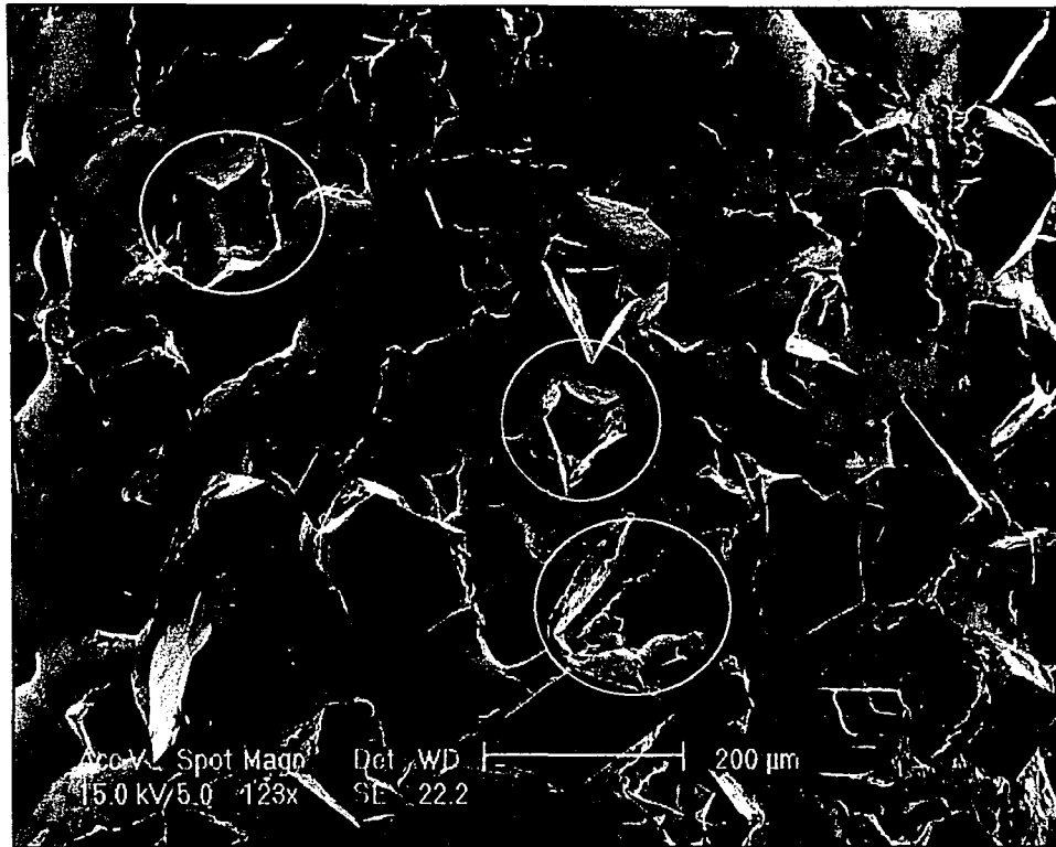
Figure 84: Clear surface of the grinding wheel used in the oil fluid trial, some abrasive grains missing on the surface are circled.
