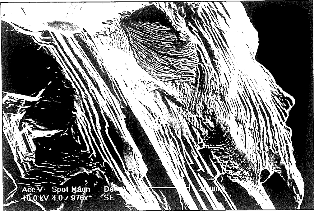
Figure 4: Morphology and scale of fine-scale structure present on fractured surfaces of CBN abrasive particles.
