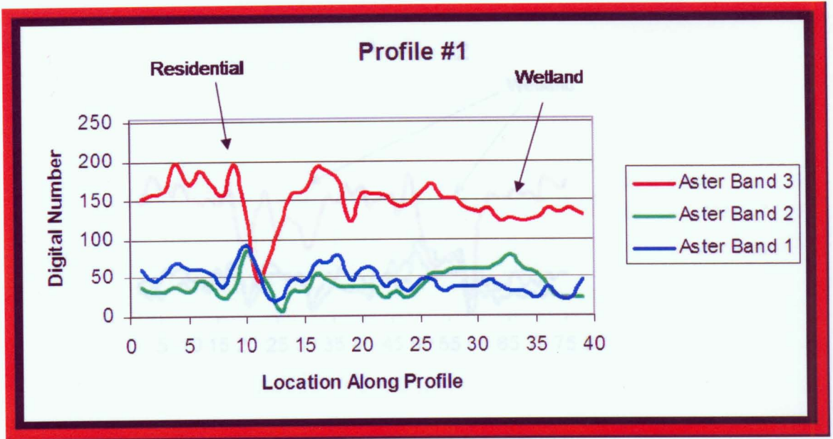
Figure 14b: Environmental spectral characteristics of the 3,2,1 Aster bands (3: near infrared, 2: visible red, and 1: visible green; spectral characteristics are relative using a digital number scheme) along transect #1 (profile values start at the transect number) where the residential area is detected as high in the visible bands and the wetland area is low in the near infrared .
